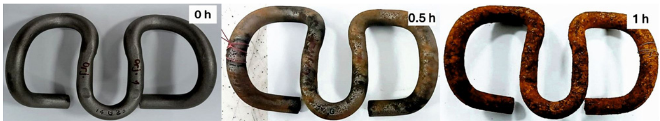
Fig. 9. Corrosion test results showing the time-based deterioration of the non-coated sample.
