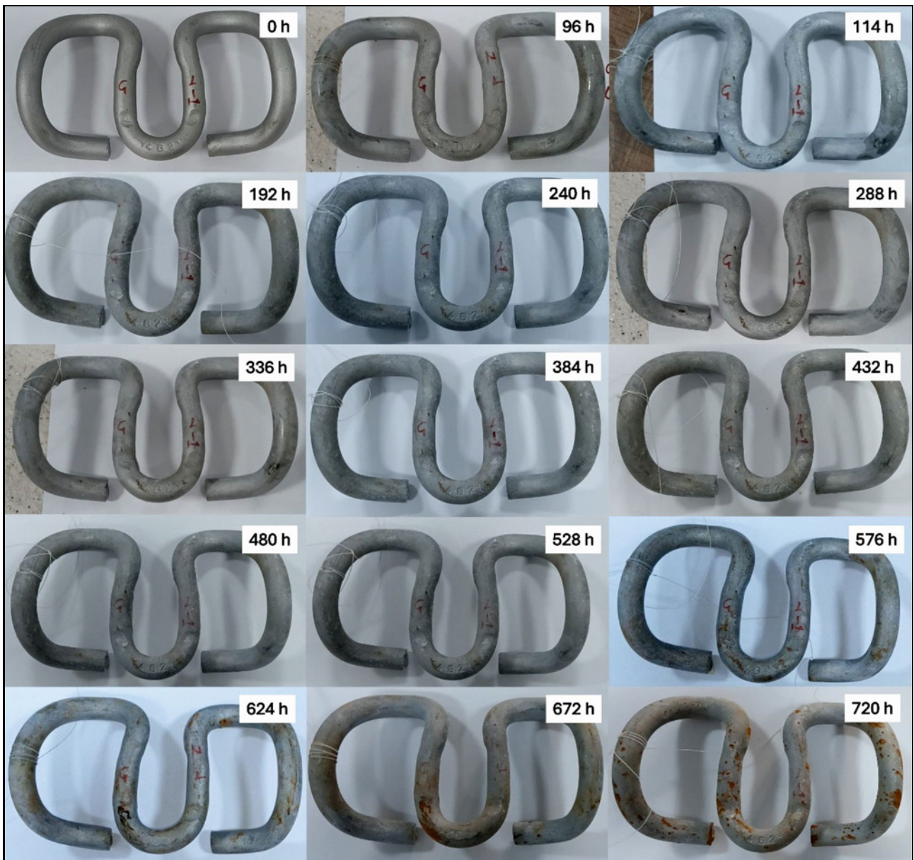
Fig. 10. Corrosion test results showing the time-based deterioration of the ZnAl-coated sample.
