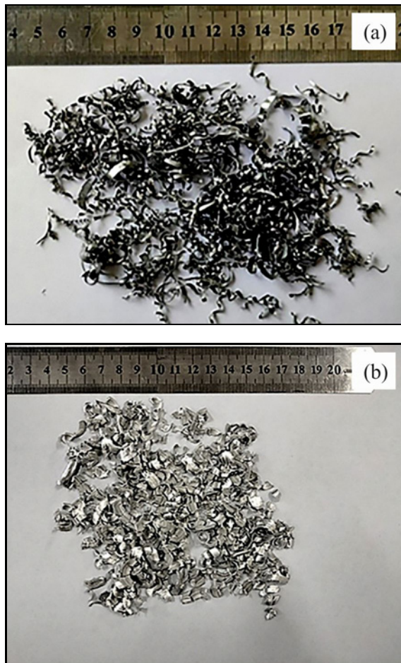
Fig. 1. Macroscopic feature of aluminium chips: (a) ADC12, and (b) 6005A.
