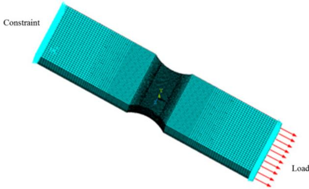
Fig. 1. Loading method for the finite element analysis model of the specimen.
