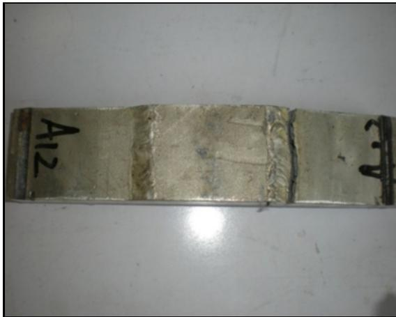
Fig. 9. The typical failure mode of the lap-welded specimen.
