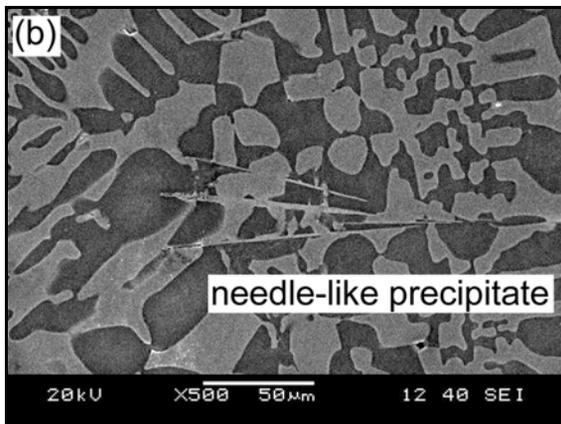
Fig. 2. Microstructure in the brazing seam region: a)  $\alpha(\text{Al})$ - $\text{CuAl}_2$  eutectic phase, b) needle-like precipitates.
