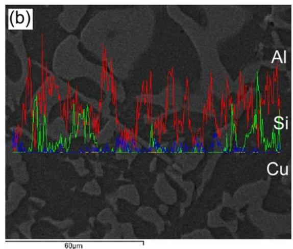
Fig. 3. Typical elements distribution in the Cu/Al brazing joint: a) elements distribution near the interface of Cu and the brazing seam region, b) elements distribution in the center of the brazing seam.
