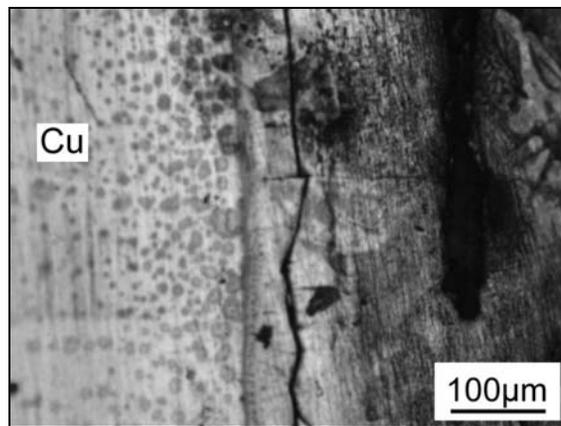
Fig. 5. Micro crack in the transition region at the Cu side.
