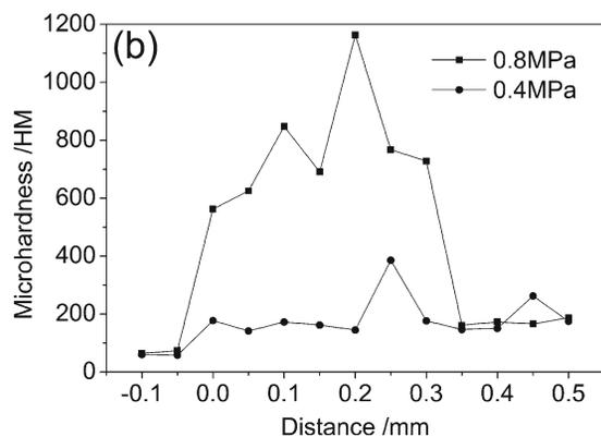
Fig. 4. Microhardness near the interface of Cu and the brazing seam region: a) testing location, b) microhardness profile.
