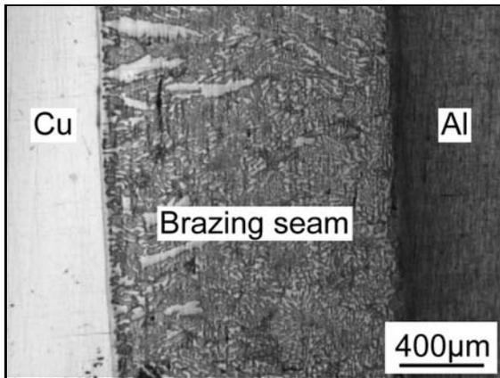
Fig. 1. Cross section of the Cu/Al brazing joint.
