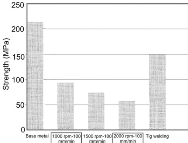
Fig. 7. Tensile strength values of the test samples.
