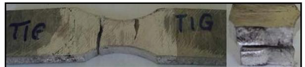
Fig. 4. Fractographs of TIG welded samples after fatigue strength test.
