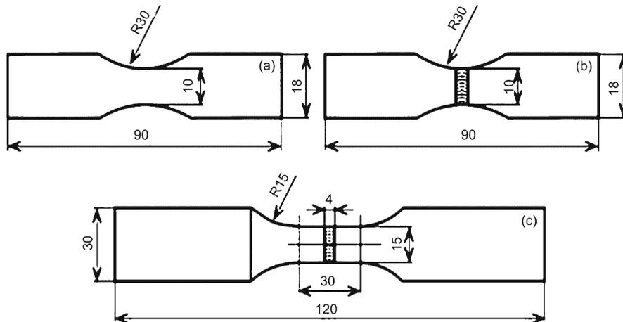
Fig. 2. a) Dimensions of fatigue base metal test specimens, b) dimensions of fatigue welding test specimens, c) tensile test samples.
