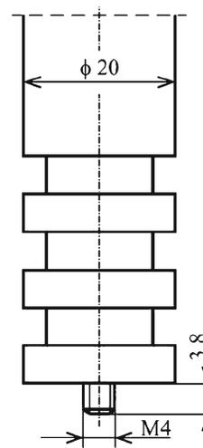
Fig. 1. Dimensions of the tool used for FSW (in mm).
