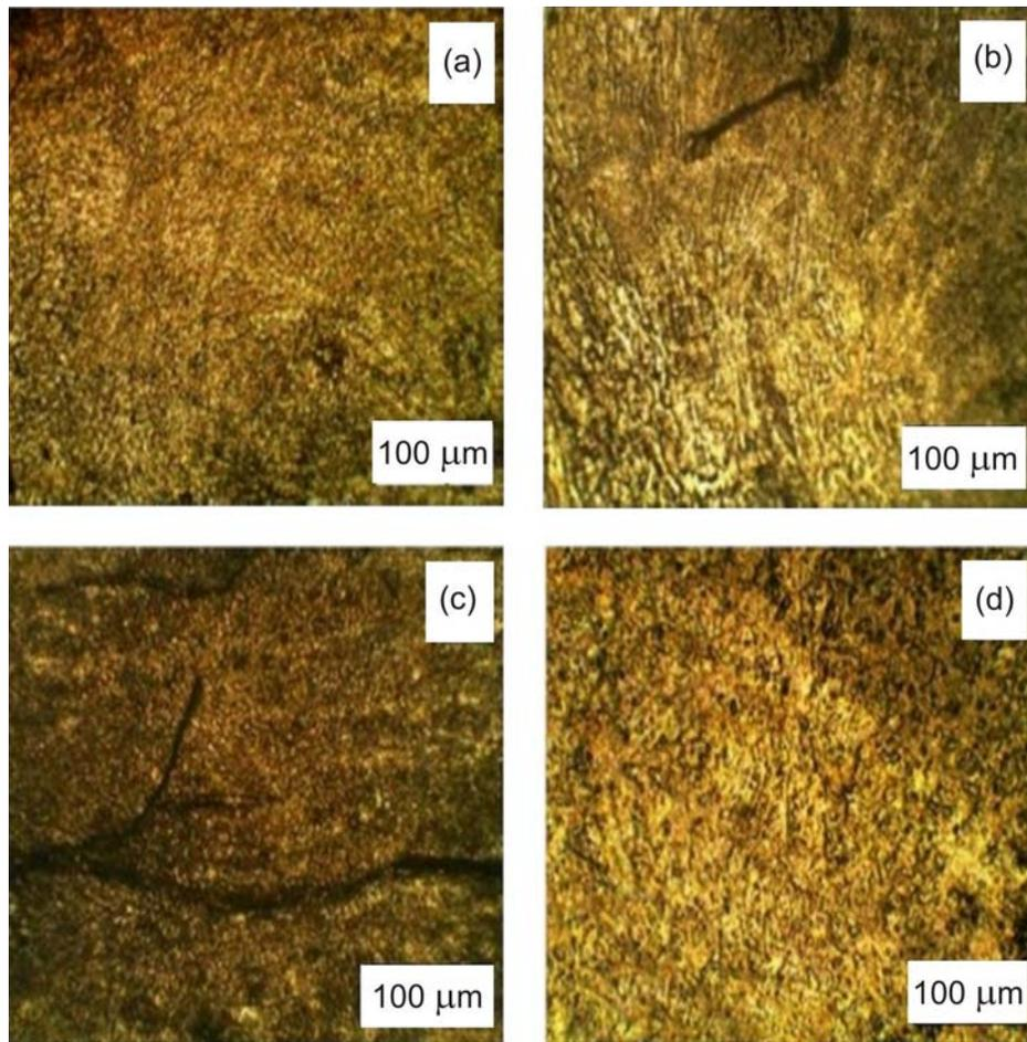
Fig. 8. Microstructures: a) 1000 rpm-100 mm min<sup>-1</sup>, b) 1500 rpm-100 mm min<sup>-1</sup>, c) 2000 rpm-100 mm min<sup>-1</sup>, d) TIG welding.
