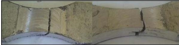
Fig. 5. Fractographs of FSWed samples.
