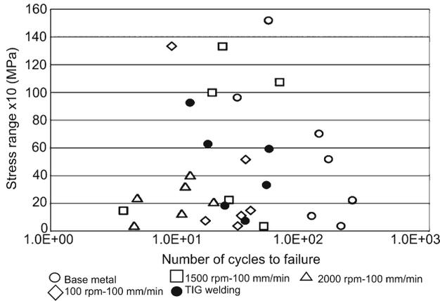
Fig. 6. Bending fatigue strength values of the test samples.
