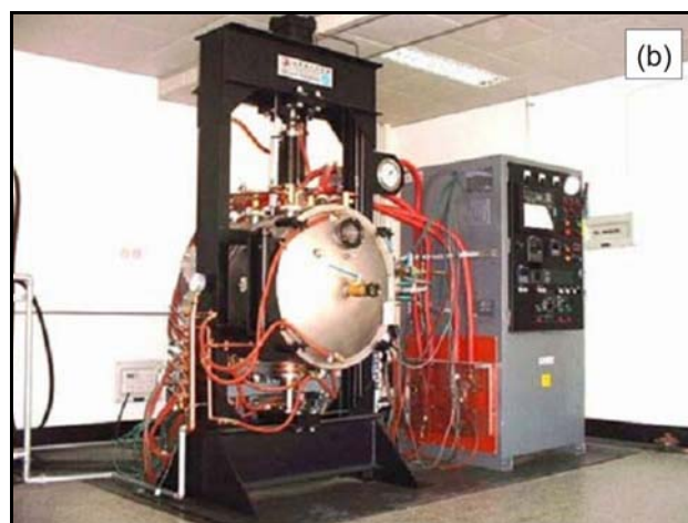
Fig. 1. Technology parameters (a) and brazing equipment (b) for vacuum brazing of Al/Cr18-Ni8 stainless steel.
