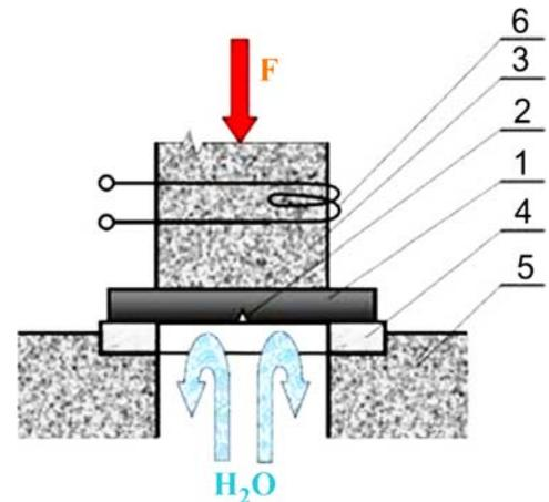
Fig. 4. The principle of cyclic thermal shocks testing method: 1 – specimen, 2 – impression, 3 – punch, 4 – sealing, 5 – support, 6 – inductor.
