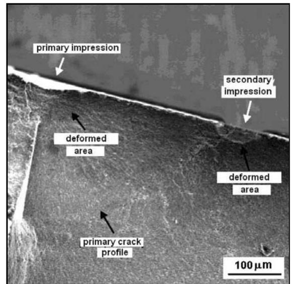
Fig. 7. Fracture surface detail, specimen No. 8, couple No. 10.
