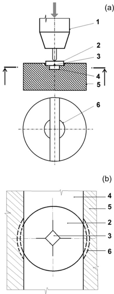
Fig. 2. The design of the fixture for the loading of the circular specimens in bending assures that the fracture occurs from the indentation cracks (a); (b) bottom view of the specimen with the indentation cracks orientation: 1 – moving element, 2 – specimen, 3 – impression, 4 – groove, 5 – static element, 6 – countersink.
