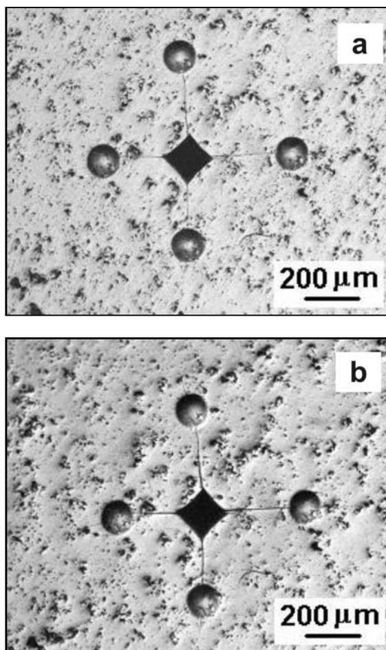
Fig. 9. Specimen with primary and secondary impressions, specimen No. 20, couple No. 10: (a) initial state, (b) after 8 cycles.
