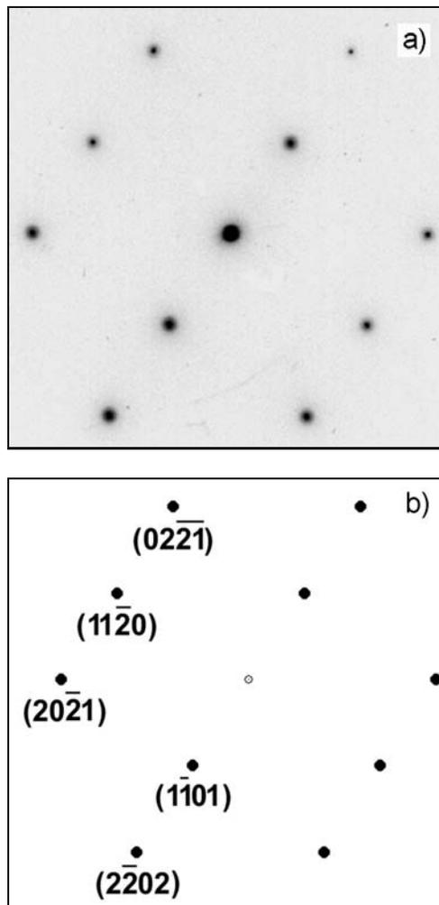
Fig. 2. Diffraction pattern from a particle containing Zn: a) compared with a simulated pattern, b) indexed unambiguously as  $[1 \ -1 \ 0 \ -2]$  pole patterns of  $\text{MgZn}_2$  hexagonal phase.
