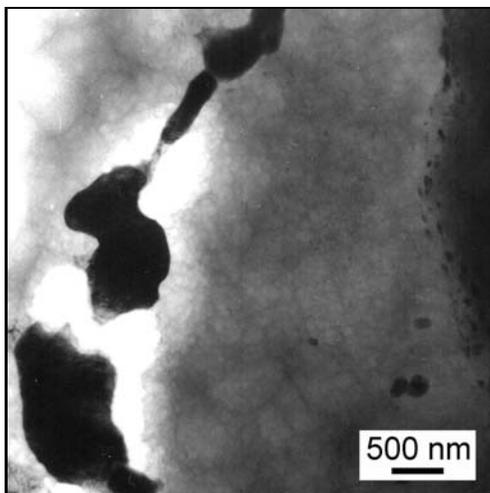
Fig. 1. Particles on grain boundary, mostly of  $\text{MgZn}_2$  phase.
