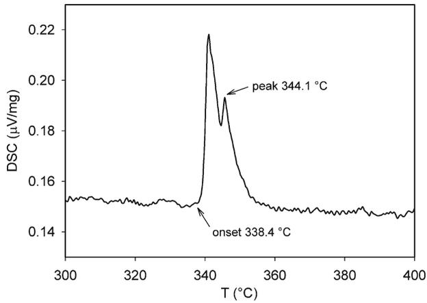
Fig. 3. DSC signal from ZK60 alloy in as-cast state.
