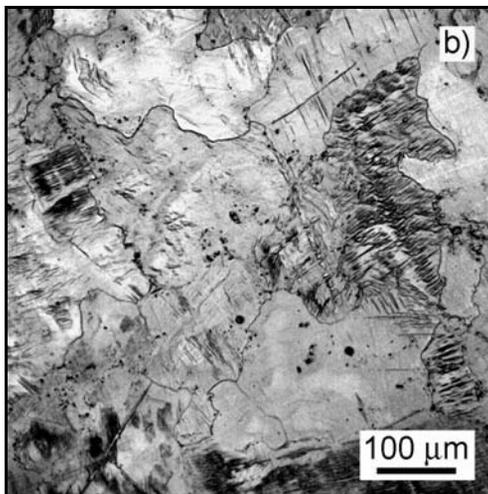
Fig. 4. The effect of annealing: a) as-received state, b) annealed 2 hours at 360 °C.
