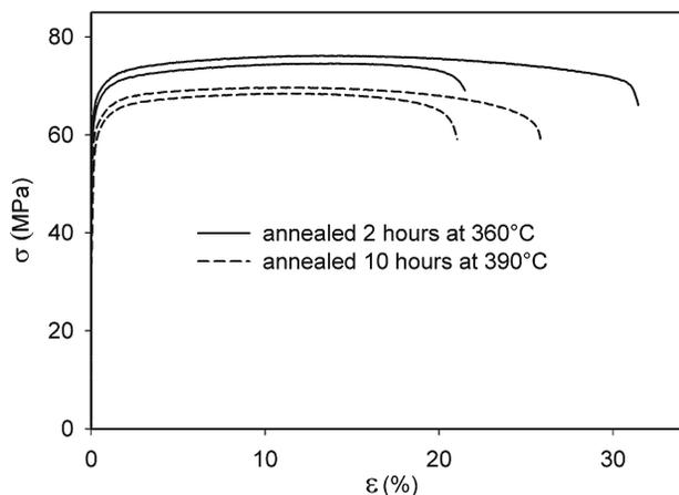
Fig. 6. Comparison of flow curves at 300°C and strain rate of  $0.05 \text{ s}^{-1}$ .
