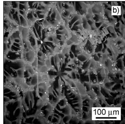
Fig. 5. SEM micrographs of samples annealed: a) 10 hours at 390 °C, b) 2 hours at 360 °C.
