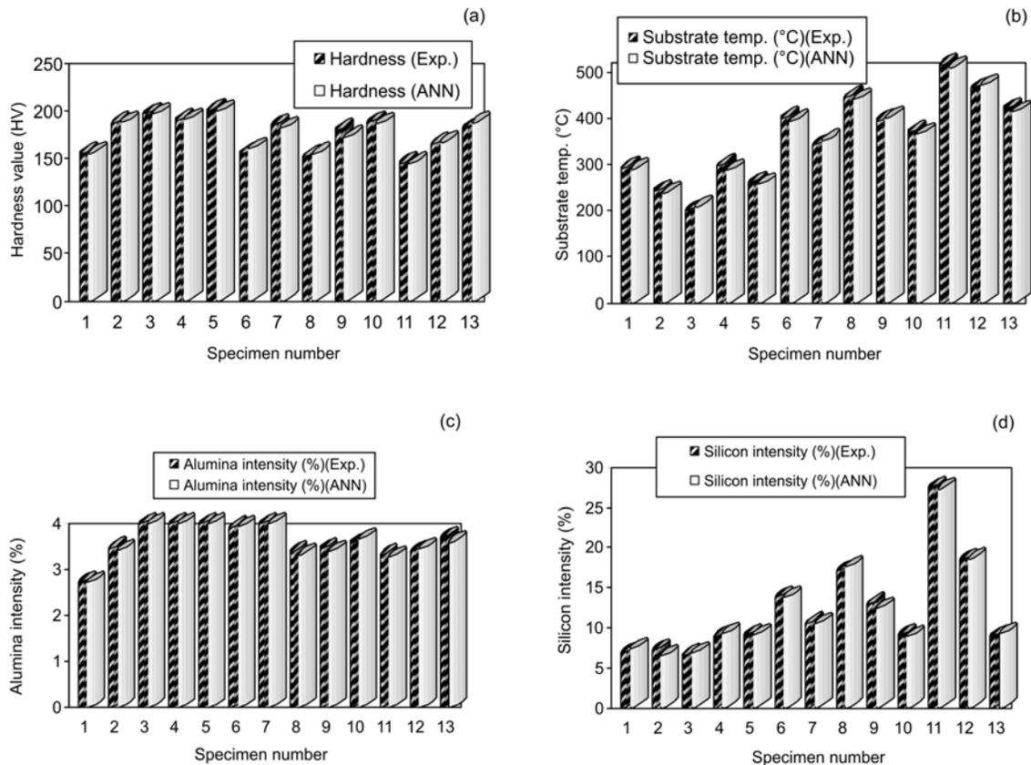
Fig. 4. The comparisons of experimental values with ANNs results at learning phase: (a) hardness, (b) substrate temperature, (c) alumina intensity, (d) silicon intensity.
