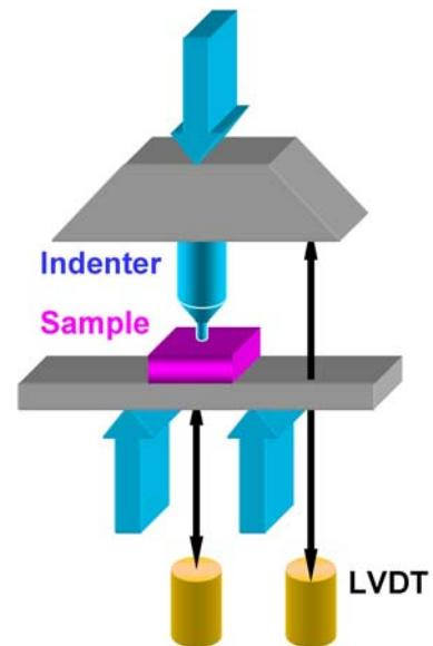
Fig. 1. Schematic illustration of the impression creep test.
