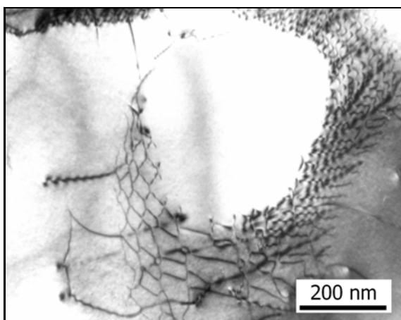
Fig. 6. Dislocation networks in MoSi<sub>2</sub> grains found after creep in bending at 1200°C.
