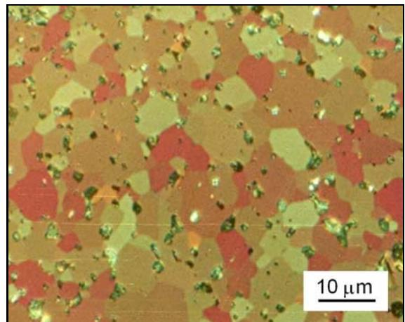
Fig. 2. Microstructure of the investigated material in cross-polarized illumination.
