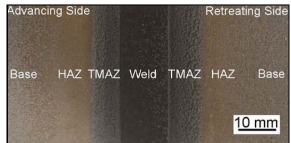
Fig. 9. Exfoliation corrosion test results.
