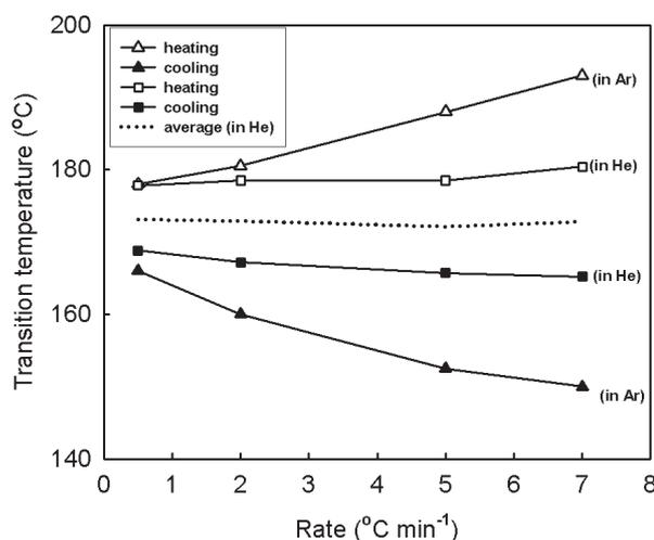
Fig. 6. Dependence of the transformation temperature on heating/cooling rate.
