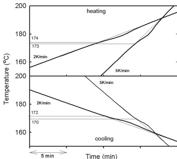
Fig. 7. Time dependence of the temperature for heating/cooling rate 2 and 5 K min<sup>-1</sup> (in He).
