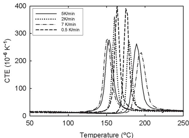
Fig. 5. Temperature dependence of the CTE for pre-deformed sample (in Ar).
