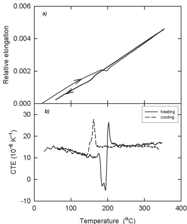
Fig. 1. Temperature dependence of the relative elongation (a) and the CTE (b) for the first thermal cycle ( $5 \text{ K min}^{-1}$  in Ar).
