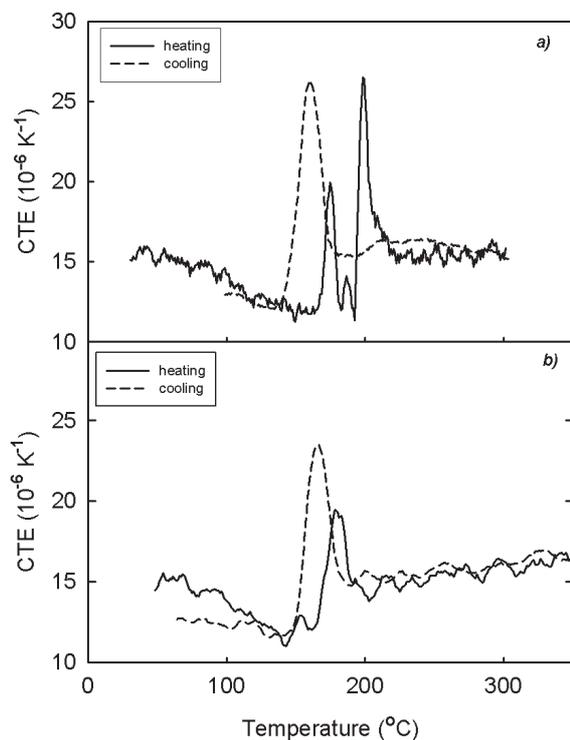
Fig. 3. Temperature dependence of the CTE (a) for the fourth thermal cycle measured by heating/cooling rate  $5 \text{ K min}^{-1}$  (b) for the second thermal cycle measured by rate  $0.5 \text{ K min}^{-1}$  (in Ar).
