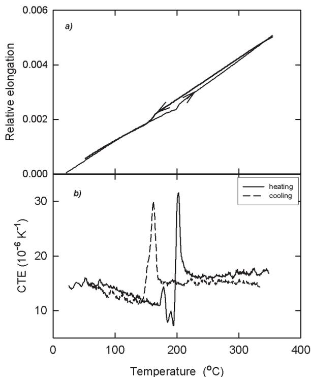
Fig. 2. Temperature dependence of the relative elongation (a) and the CTE (b) for the second thermal cycle ( $5 \text{ K min}^{-1}$  in Ar).
