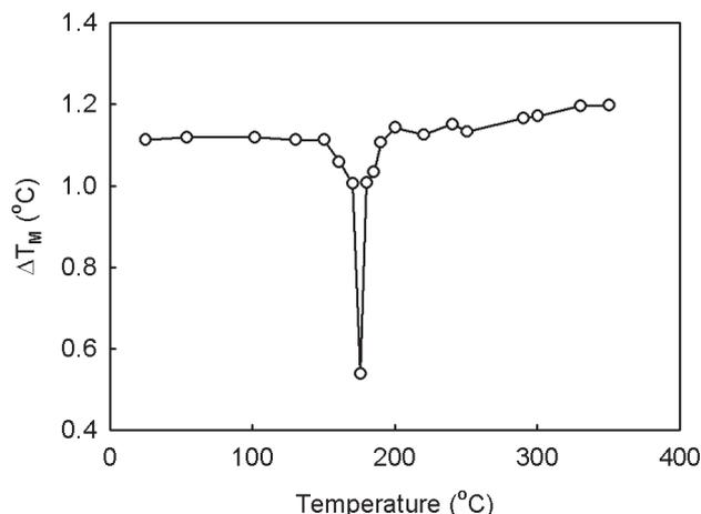
Fig. 9. Temperature dependence of the maximum temperature rise of the sample irradiated by pulse of energy in the flash method.
