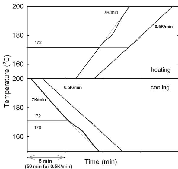
Fig. 8. Time dependence of the temperature for heating/cooling rate 0.5 and 7 K min<sup>-1</sup> (in He).
