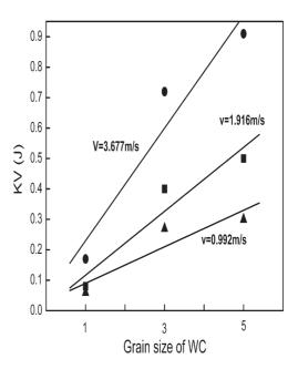
Fig. 3. Effect of the grain size of WC grains on the impact energy of WC-Co materials at different velocities.
