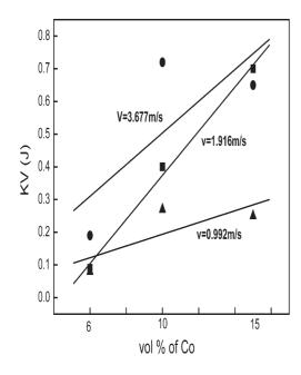
Fig. 4. Effect of the vol.% of Co on the impact energy of WC-Co materials at different velocities.
