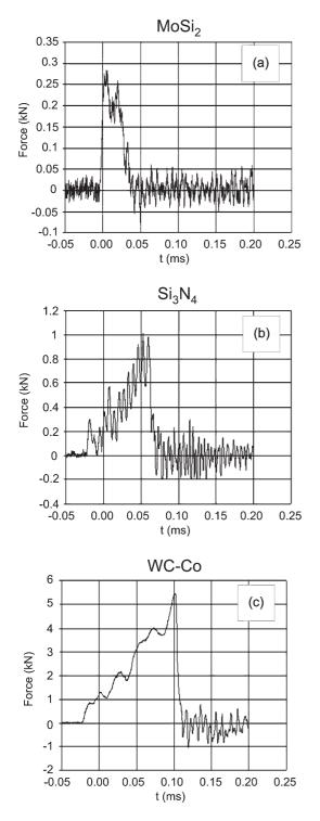
Fig. 1. Force signal for  $MoSi_2$  (a),  $Si_3N_4$  (b), and WC-Co (c).
