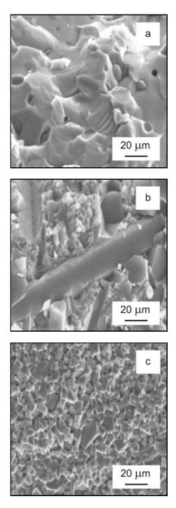
Fig. 5. Fracture surface of the MoSi<sub>2</sub> (a), Si<sub>3</sub>N<sub>4</sub> (b), and WC-Co (c) after Charpy test.
