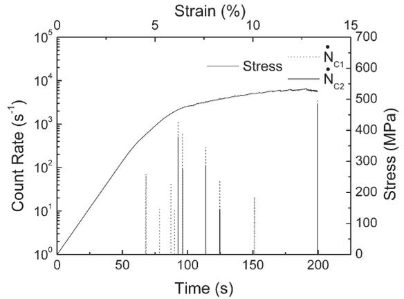
Fig. 6. Stress-strain and AE count rate-time curves of 1441 alloy, position 3.
