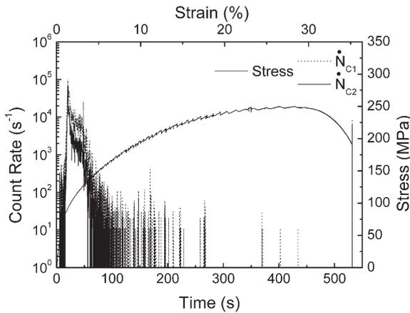
Fig. 4. Stress-strain and AE count rate-time curves of 5754 alloy, position 4.
