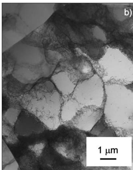
Fig. 5. TEM micrograph of subgrain structure (a) and dislocation cell structure (b) formed in the flat area of the grooved plate (segment 1-A-TEM).
