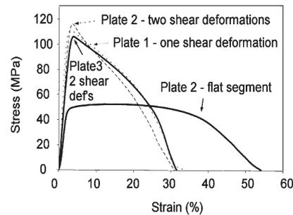
Fig. 14. Records of tensile tests performed with small specimens for different segments of plates.
