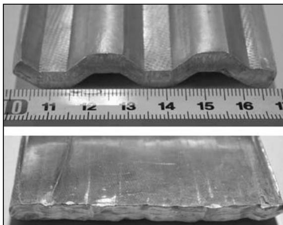
Fig. 3. The deformed plate shape after the pressing and straightening.
