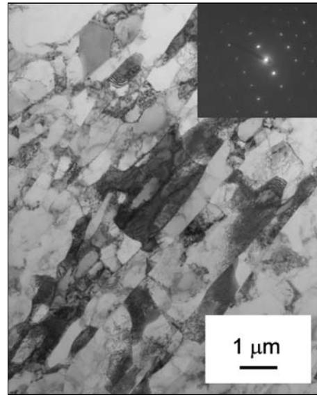
Fig. 7. TEM micrograph showing the subgrain formation in sheared region (1-B-TEM).
