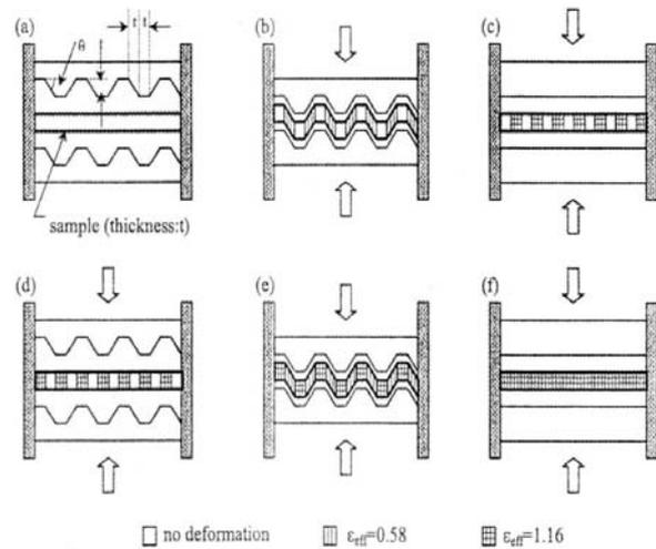
Fig. 2. A schematic illustration of CGP method [1].
