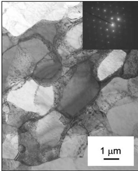
Fig. 9. TEM micrograph formation of new grains with high angle boundaries (2-B-TEM specimen).
