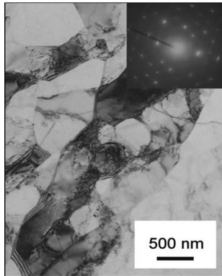
Fig. 8. TEM micrograph of polygonized structure (1-B-TEM specimen).
