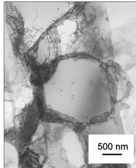
Fig. 12. Formation of new grains by dislocation re-arrangement (3-A-TEM).
