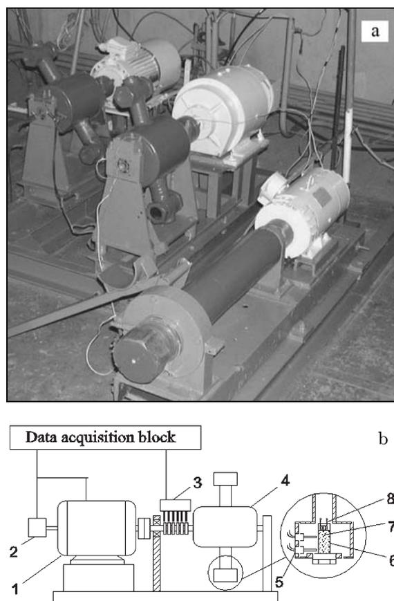
Fig. 1. Outside view (a) and sketch (b) of the centrifugal machine used in experiments: (1) electric motor, (2) tachometer, (3) collector, (4) rotor, (5) photodiodes, (6) quartz mould, (7) sample, (8) igniter.
