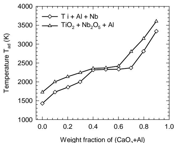
Fig. 2. Dependence of calculated  $T_{ad}$  on relative weight fraction of energy-producing component ( $\nu_2$ ).
