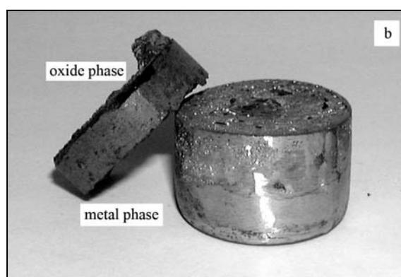
Fig. 4. Outward appearance of the ingot before (a) and after (b) separation of the oxide layer from the metallic part.
