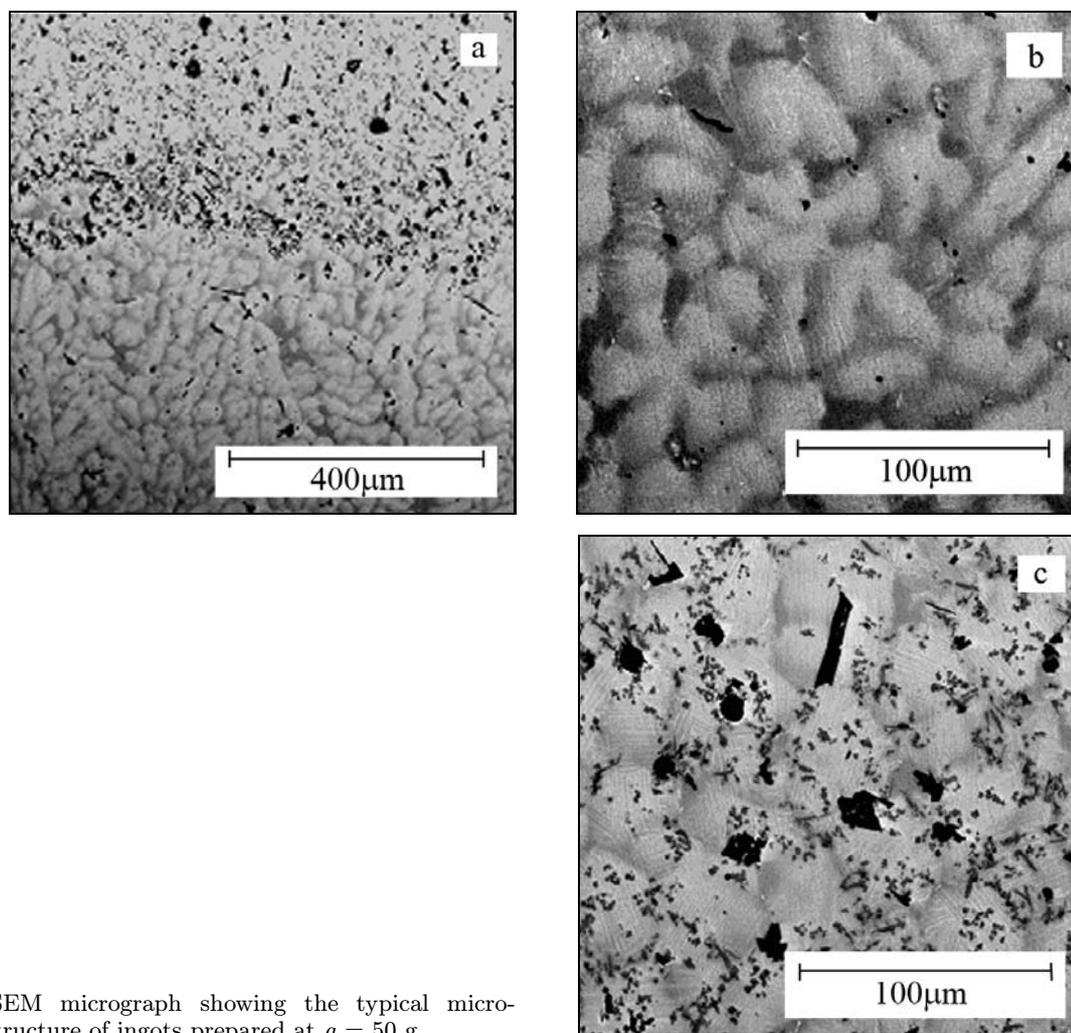
Fig. 6. SEM micrograph showing the typical microstructure of ingots prepared at  $a = 50$  g.
