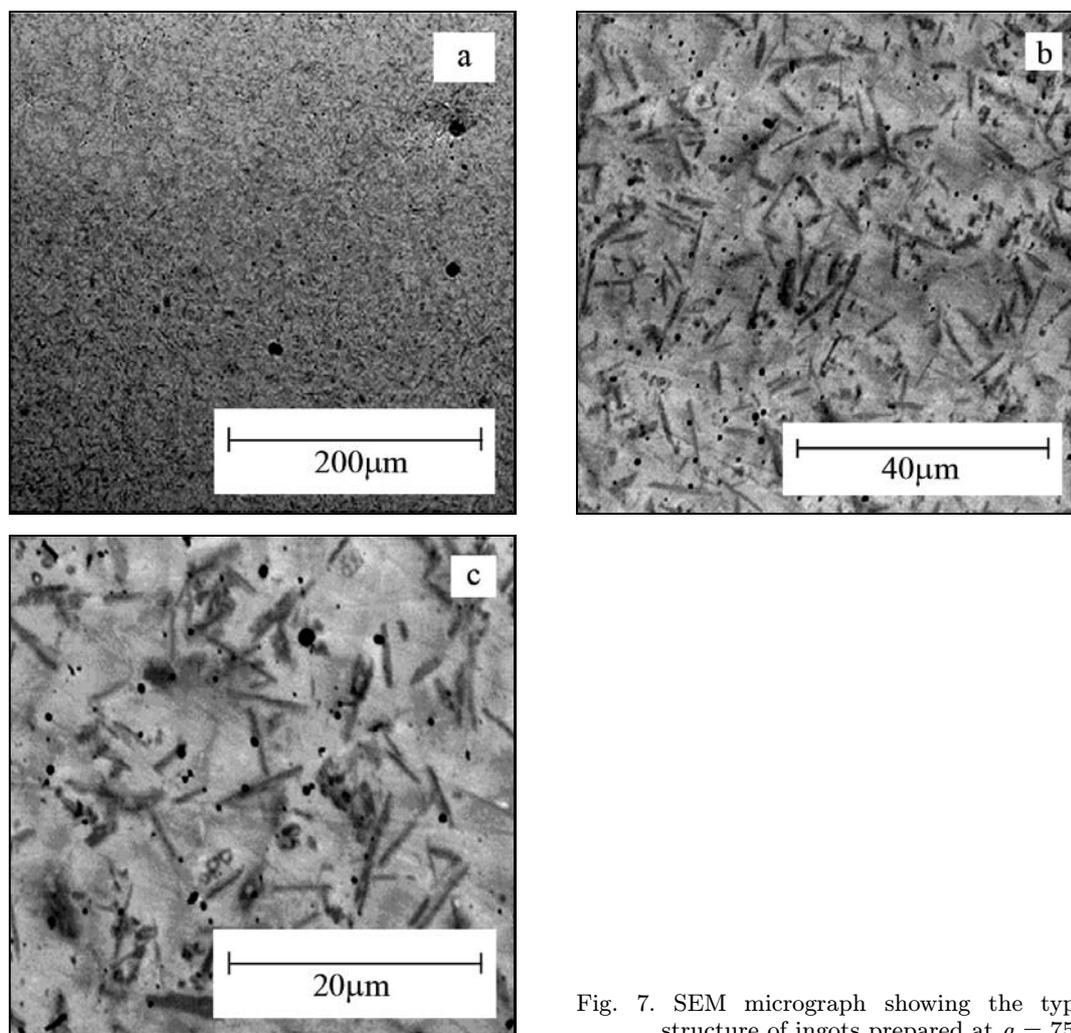
Fig. 7. SEM micrograph showing the typical microstructure of ingots prepared at  $a = 750$  g.
