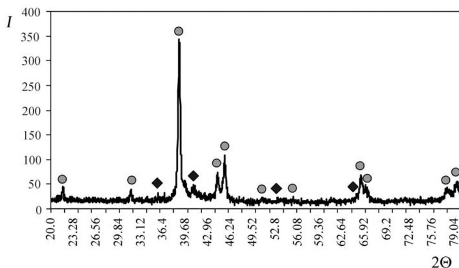
Fig. 5. The typical diffraction pattern of metallic part of ingots produced by SHS: (◆) Ti<sub>3</sub>Al and (●) TiAl.
