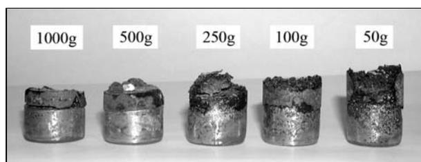
Fig. 3. Photographs showing ingots prepared by SHS in centrifugal machine at various centrifugal acceleration  $a$ .
