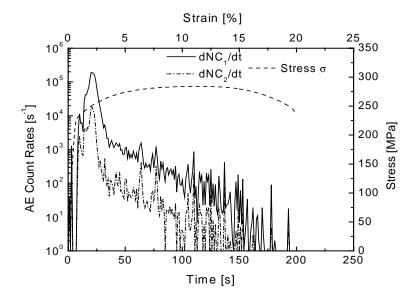
Fig. 4. Stress-strain and AE count rates-time curves for extruded AZ31 alloy with grain size 6  $\mu {\rm m}.$
