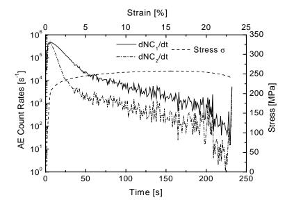
Fig. 6. Stress-strain and AE count rates-time curves for extruded AZ31 alloy with grain size 22  $\mu$ m.
