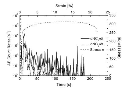
Fig. 3. Stress-strain and AE count rates-time curves for extruded AZ31 alloy with grain size 4  $\mu{\rm m}.$
