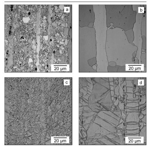
Fig. 1. Micrographs of extruded AZ31 alloy: (a) hydrostatic, grain size 4  $\mu$ m, (b) indirect, grain size 22  $\mu$ m, (c) hydrostatic, grain size 4  $\mu$ m, after tensile testing, (d) indirect, grain size 22  $\mu$ m, after tensile testing.
