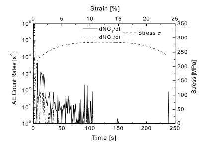
Fig. 5. Stress-strain and AE count rates-time curves for extruded AZ31 alloy with grain size 8  $\mu {\rm m}.$
