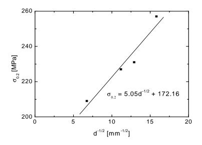
Fig. 2. The dependence of the yield strength  $\sigma_{0.2}$  on the  $d^{-1/2}$ .
