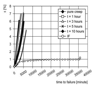
Fig. 3. Strain-time to failure dependences for longer holds.
