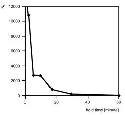
Fig. 5. Plot of the time to failure in terms of the sum of hold time at maximum load.
