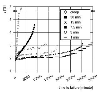
Fig. 4. Strain-time to failure dependences for shorter holds.
