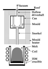
Fig. 10. Schematic view of the equipment used for counter-gravity casting TiAl components.
