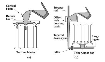
Fig. 6. Schematic mould designs for casting turbine blades using (a) top-gating and (b) bottom-gating.
