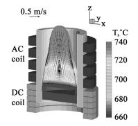
Fig. 5. Effect of superimposing a DC field (10 kA) on the flow and temperature in a 2.8 kg charge of Al alloy.
