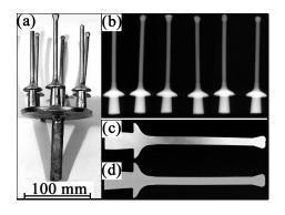
Fig. 11. (a) Mould of counter-gravity cast Al valves; (b) radiograph showing absence of defects; (c) polished macro-section; (d) etched macro-section.
