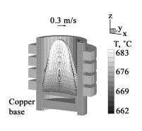
Fig. 4. Example of simulation of ISM furnace. 2.8 kg Al alloy melted with 5560 A coil current.
