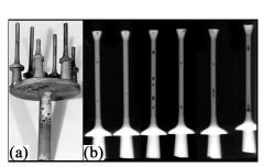
Fig. 12. Counter-gravity cast TiAl valves:(a) incompletely-filled mould due to too low a differential pressure; (b) radiograph showing turbulence-induced bubbles due to too high a differential pressure.
