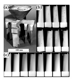
Fig. 9. (a) Top-gated mould of TiAl turbine blades; (b) many small bubbles formed with a mould temperature of 1000  $^{\circ}$ C; (c) much improved quality with a mould temperature of 1300  $^{\circ}$ C.
