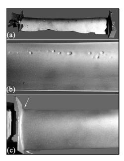
Fig. 1. Typical defects in commercial TiAl castings: (a) misrun; (b) HIP sinks; (c) cracks.
