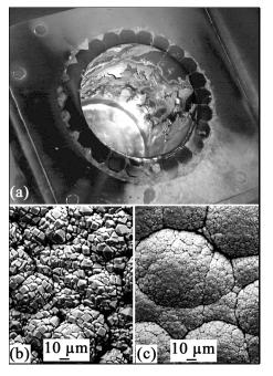
Fig. 3. (a) Deposits on ISM crucible after melting TiAl under vacuum; (b) SEM image of one area: 49 % Al, 42 % O, 8 % Mn (wt.%); (c) SEM image of another area: 85 % Al, 12 % Mn (wt.%).
