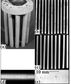
Fig. 7. (a) Typical top-gated mould used to cast 20 mm diameter bars (the pouring bush is missing); (b) isolated bubbles in bars cast in mould at 500 °C; (c) absence of major defects in bars cast in mould at 1000 °C; (d) radiograph and (e) macrosection showing layer porosity.
