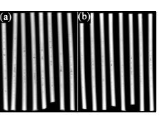
Fig. 14. 10 mm diameter TiAl bars centrifugally-cast in a multi-layer mould showing defects in (a) top layer; (b) bottom layer.
