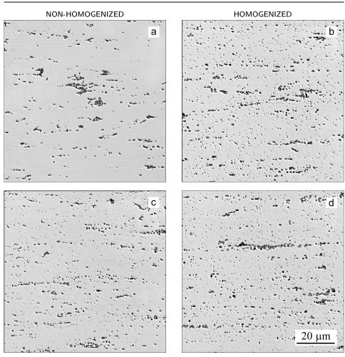
Fig. 2. Second-phase particles in non-homogenized (a) (c) and homogenized (b) (d) sheets of the AlMg2Mn0.8 (AA5049) alloy at the final gauge 1.0 mm.
