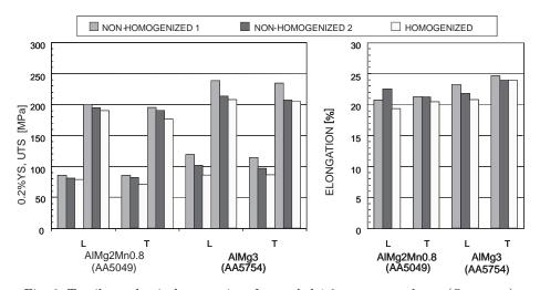
Fig. 6. Tensile mechanical properties of annealed 1.0 mm gauge sheets (O-temper).
