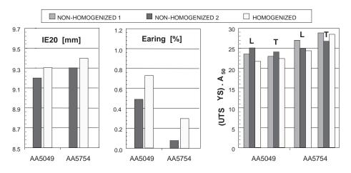
Fig. 7. Height of Erichsen dome (IE20), results of the cupping test (Earing) and formability parameter (UTS-YS).A50 of annealed 1.0 mm gauge sheets (O-temper).
