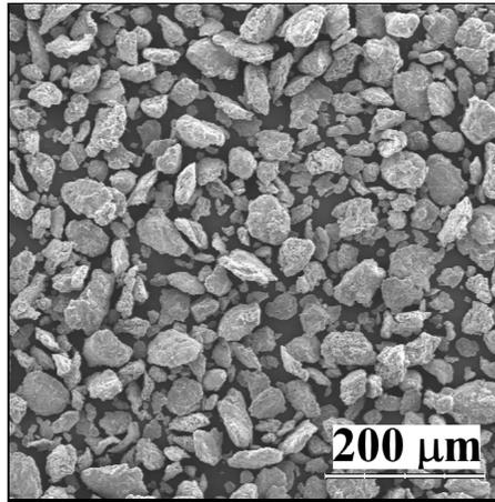
Fig. 3. Secondary electron micrograph of as-milled NiAl30 powder (SEM).
