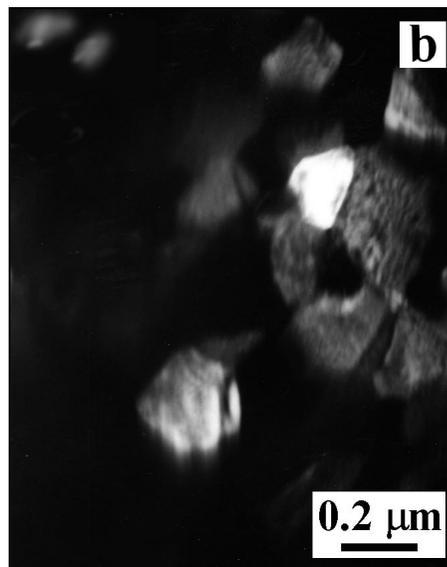
Fig. 10b. Dark field image formed using the (101) reflection of  $\beta$ -NiAl.
