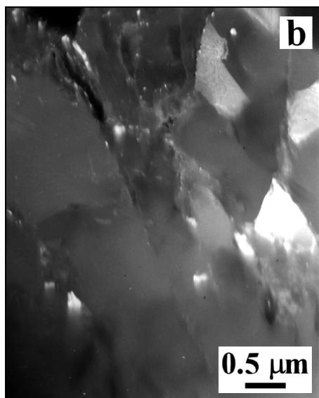
Fig. 7b. Dark field image formed using  $(\bar{1}11)$  reflection of Al.
