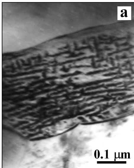
Fig. 9a.  $\beta$ -NiAl in the microstructure of NiAl30 powder (TEM, BF image).
