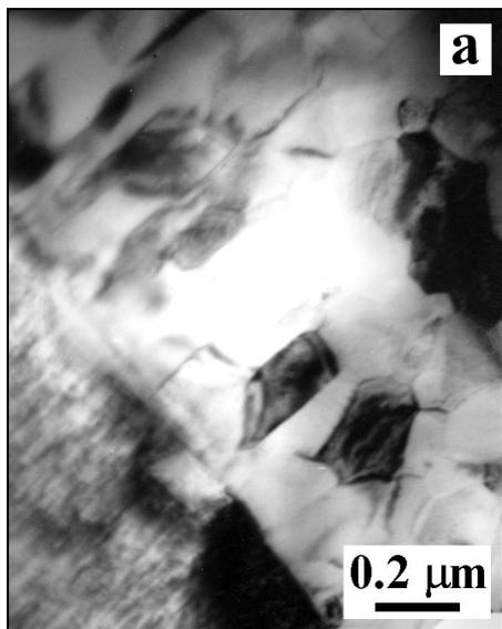
Fig. 10a. Fine grained  $\beta$ -NiAl in the microstructure of NiAl30 powder (TEM, BF image).
