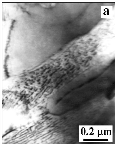
Fig. 8a.  $\beta$ -NiAl phase with mottled appearance in the microstructure of NiAl30 powder (TEM, BF image).
