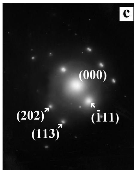
Fig. 7c. SAED pattern corresponding to  $[\bar{1}21]$  zone of Al.
