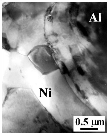
Fig. 6. Interlayer boundary region in the microstructure of as-milled NiAl30 powder (TEM, BF image).
