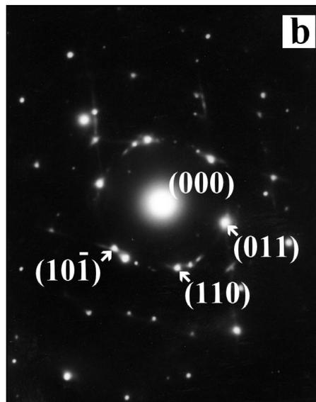
Fig. 9b. SAED pattern corresponding to  $[1\bar{1}1]$  zone of  $\beta$ -NiAl.
