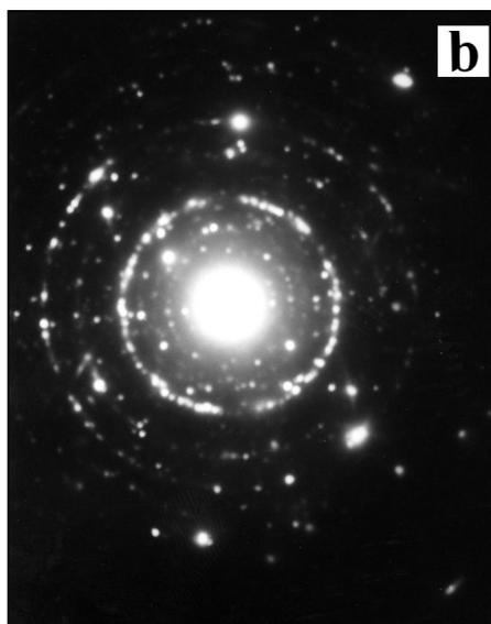
Fig. 11b. SAED ring pattern corresponding to random orientation of  $\text{Ni}_2\text{Al}_3$ .
