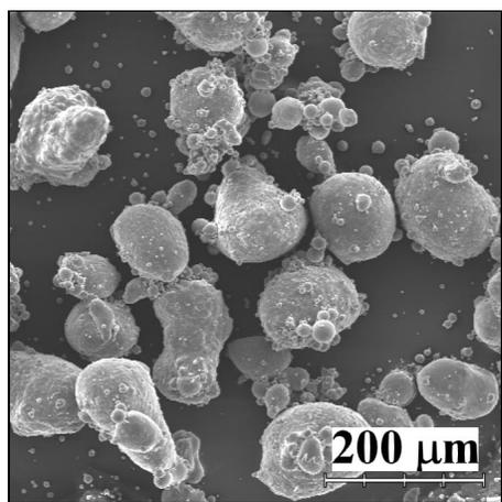
Fig. 1. Secondary electron micrograph of the initial Al powder (SEM).
