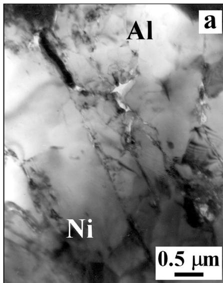
Fig. 7a. Interlayer boundary region in the microstructure of as-milled NiAl30 powder (TEM, BF image).
