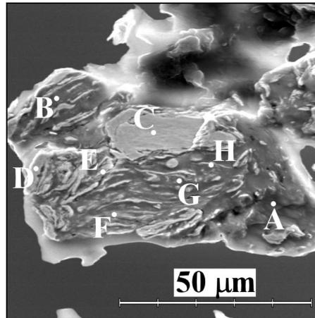
Fig. 5. Microstructure of NiAl30 powder as observed in the particle cross-section (SEM).
