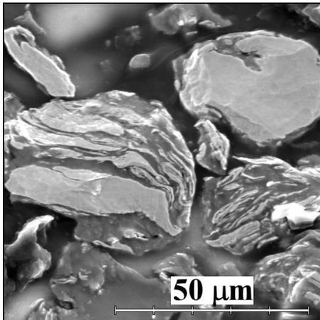
Fig. 4. Secondary electron micrograph of the cross-section of NiAl30 powder (SEM).
