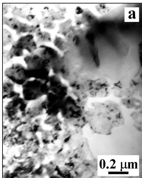
Fig. 11a. Nanocrystalline  $\text{Ni}_2\text{Al}_3$  in the microstructure of  $\text{NiAl}_{30}$  powder (TEM, BF image).
