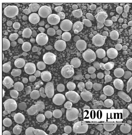
Fig. 2. Secondary electron micrograph of initial Ni powder (SEM).
