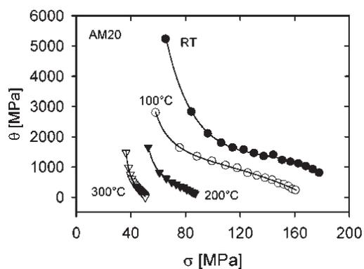
Fig. 2. Stress dependence of the work hardening rate; experimental data (points) fitted by the predicted equation (solid lines).
