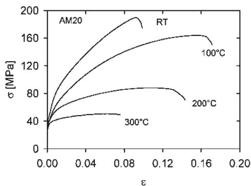
Fig. 1. True stress-true strain curves of AM20 polycrystals deformed at  $6.2 \times 10^{-5} \text{ s}^{-1}$  at various temperatures.
