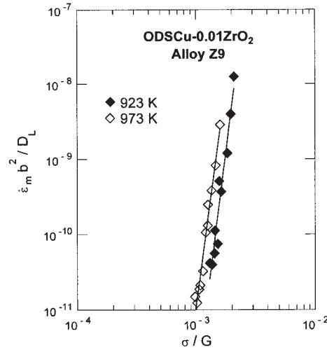
Fig. 4. Relations between the normalized creep strain rates  $\dot{\varepsilon}_m b^2 / D_L$  and the normalized applied stresses  $\sigma / G$  in double logarithmic co-ordinates.
