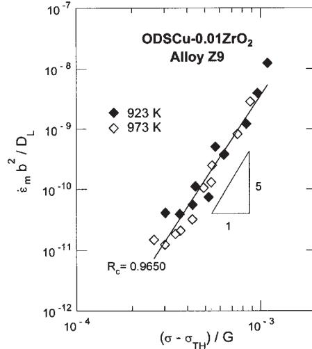
Fig. 3. The normalized minimum creep strain rates  $\dot{\varepsilon}_m b^2 / D_L$  plotted against normalized effective stresses  $(\sigma - \sigma_{TH}) / G$  in double logarithmic co-ordinates. The data points can be fitted by a single straight line, the slope of this line is close to the value of the true stress exponent  $n = 5$ .
