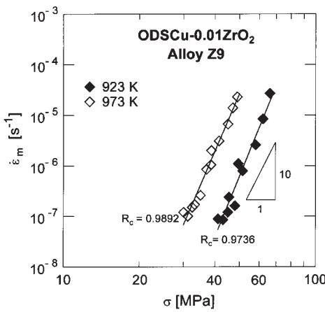
Fig. 1. Relations between minimum creep strain rates  $\dot{\varepsilon}_m$  and applied stresses  $\sigma$  for temperatures 923 and 973 K in double logarithmic co-ordinates.  $R_c$  means the correlation coefficient. Data after Nagorka et al. [8] (see Table 1).
