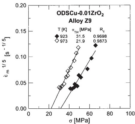
Fig. 2. Relations between  $\dot{\varepsilon}_m^{1/n}$  vs.  $\sigma$  in double linear co-ordinates. The true stress exponent of creep strain rate,  $n$ , is taken equal to 5 (cf. Ref. [9]).
