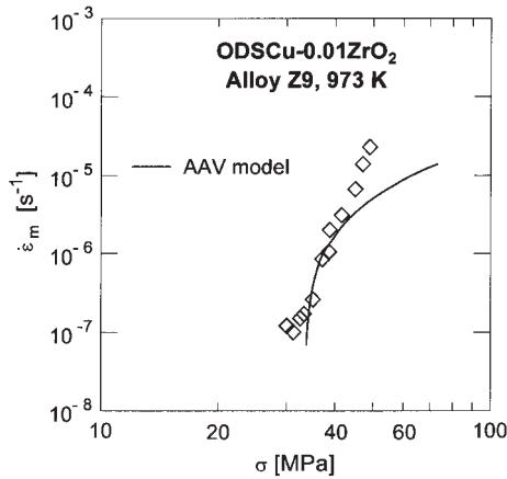
Fig. 6. The  $\dot{\varepsilon}_m(\sigma, T)$  creep data presented in the double logarithmic  $\dot{\varepsilon}_m$  vs.  $\sigma$  co-ordinates compared with the prediction of the Arzt-Ashby-Verrall (AAV) model of diffusional creep inhibited by fine particles located at grain boundaries (after Nagorka et al. [8]).
