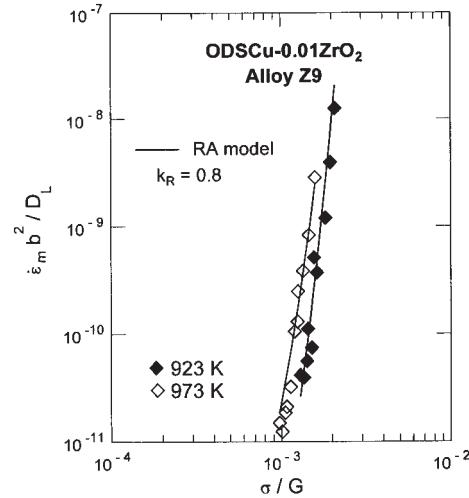
Fig. 5. Comparison of the Rösler-Arzt model with the experimental creep data. The relaxation factor  $k_R$  independent of temperature and equal to 0.80 is accepted.
