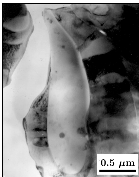
Fig. 10. Amorphous oxide inclusion in the microstructure of NiAl coating (TEM, BF image).
