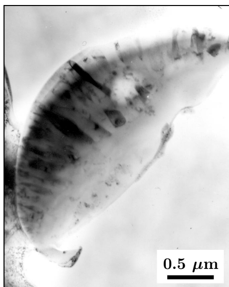
Fig. 9. Partially crystallized oxide inclusion in the microstructure of NiAl coating (TEM, BF image).
