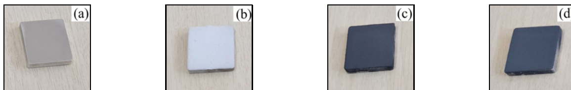
Fig. 1. Test materials (AA 5083): (a) uncoated, (b) AT0 coated, (c) AT13 coated, and (d) AT40 coated.
