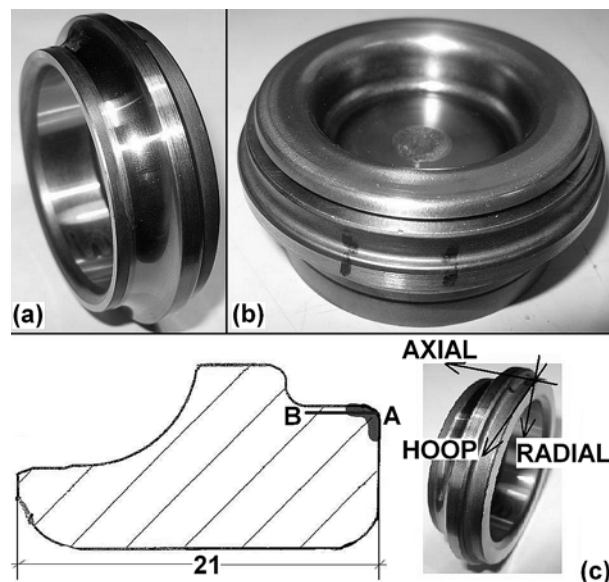
Fig. 1. Investigated rings and measurement details: free ring after manufacture (a), ring with the hub introduced (b), measurement stress components (c). Marked dimension is in mm.
