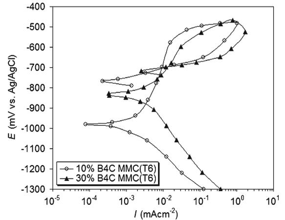
Fig. 4. CP curves of aged composites in deaerated solution.
