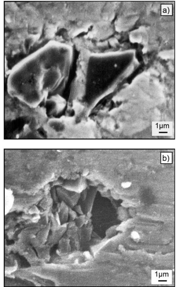
Fig. 6. a) Preferential corrosion formed around B<sub>4</sub>C particles in the 10 vol.% B<sub>4</sub>C composite and b) established pit on the 30 vol.% B<sub>4</sub>C composite in the T6 conditions.
