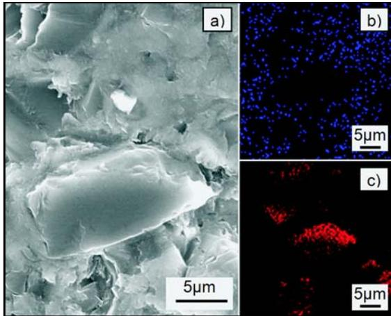
Fig. 8. a) SEM image and the X-ray maps of b) Cu and c) B of 30 vol.% B<sub>4</sub>C composite.
