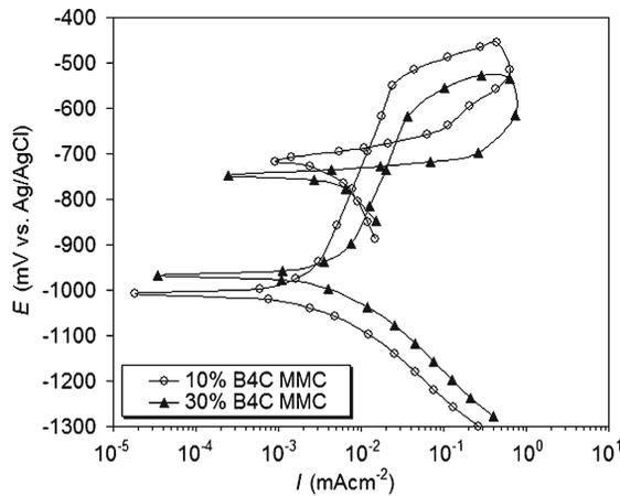
Fig. 3. CP curves of unaged composites in deaerated solution.
