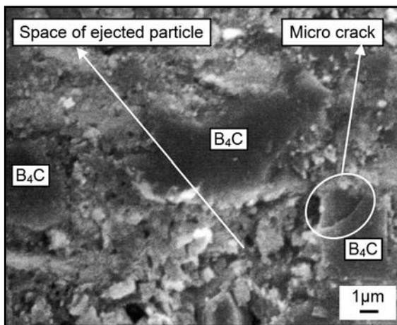
Fig. 9. Micro-cracks and dispossed place of boron carbide due to intensive matrix corrosion in T6 heat-treated 30 vol.% B<sub>4</sub>C composite.
