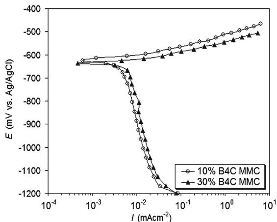
Fig. 1. PDS curves of unaged composites in aerated solution.
