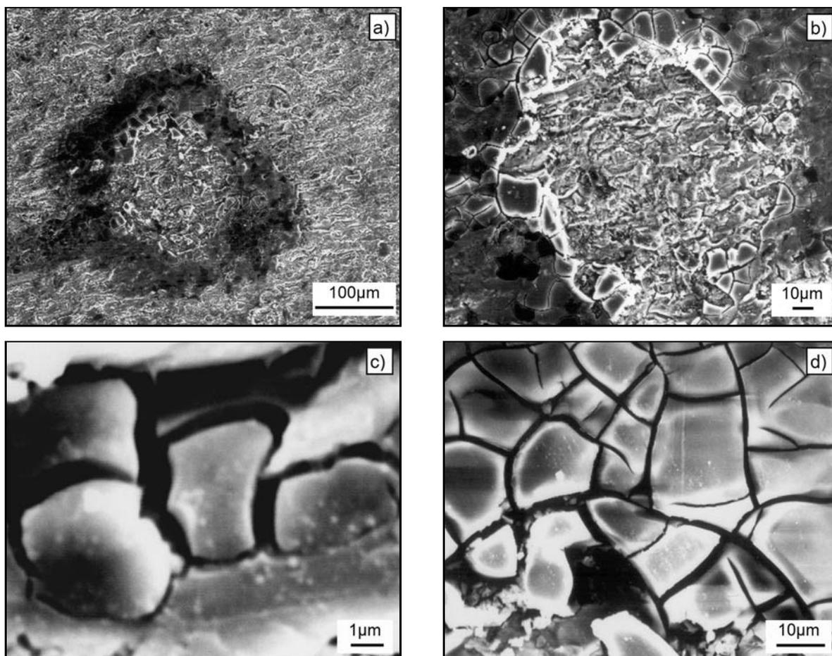
Fig. 10. Micro-submicro local batteries in a) the 10 vol.% and b) 30 vol.%  $B_4C$  composites and typical oxide micrographs of c) the 10 vol.% and d) 30 vol.%  $B_4C$  composites.
