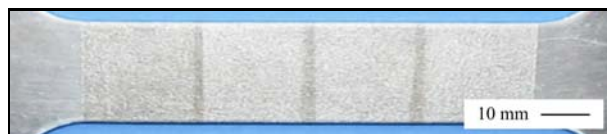
Fig. 3. The shot-peened specimen surface.
