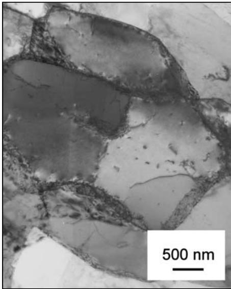
Fig. 6. TEM micrograph of high-angle grain boundaries formation on subgrains (1-B-TEM).
