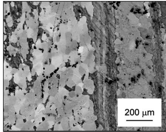
Fig. 1. LOM micrograph of initial recrystallized structure of aluminium.
