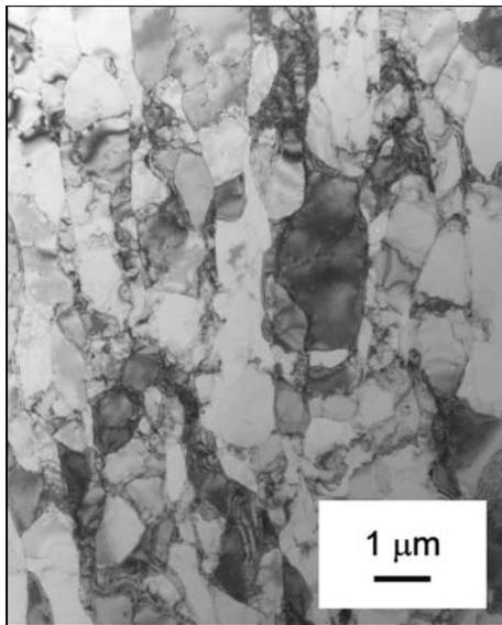
Fig. 10. TEM micrograph of subgrains microstructure after second pressing between grooved dies (3-A-TEM).
