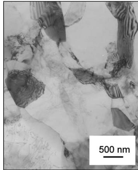
Fig. 11. New high angle grains formed on former subgrains (3-A-TEM).
