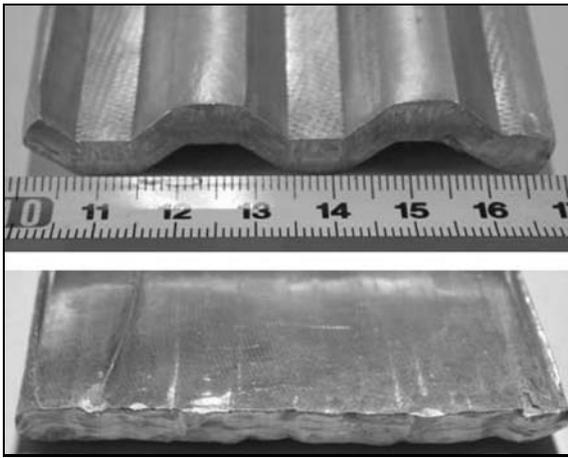
Fig. 3. The deformed plate shape after the pressing and straightening.
