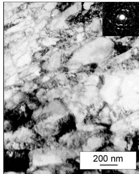
Fig. 6. Different size of fragmented ferrite subgrains produced at ECAP of 150^\circ\text{C} .
