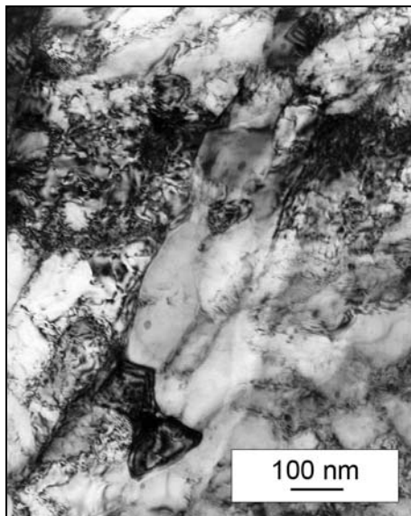
Fig. 7. TEM micrograph of new subgrains formation at ECAP temperature of 200°C.
