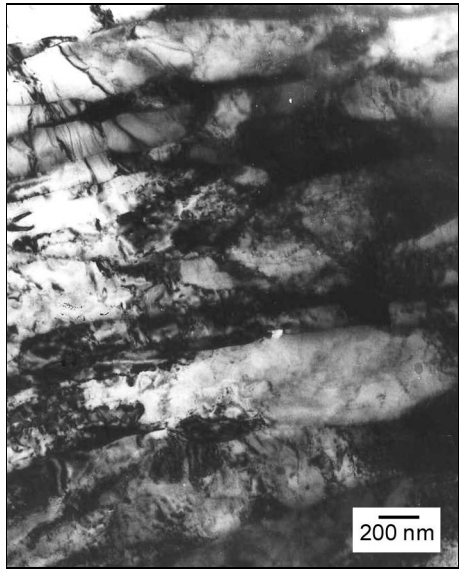
Fig. 5. TEM micrograph of as-pressed microstructure of array of deformed ferrite consisting of elongated grains produced by one pass.
