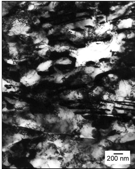
Fig. 9. TEM micrograph showing the substructure in ECAPed specimen subjected to two passes.
