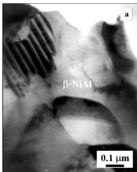
Fig. 6a. Plate-like martensitic NiAl neighbouring \beta -NiAl (TEM, BF image).
