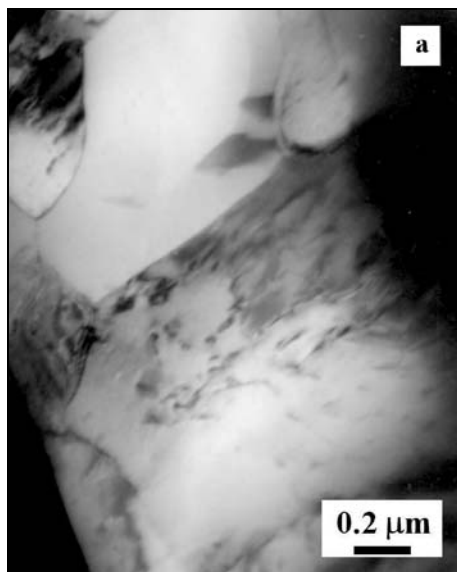
Fig. 8a. \beta -NiAl grain with small \text{Al}_3\text{Ni} particles (TEM, BF image).
