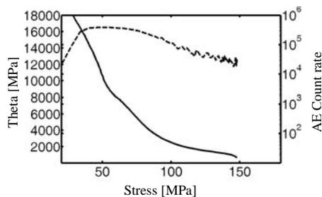
Fig. 5. Strain hardening rate vs. stress (—) and AE (---) for squeeze-cast AS21X.
