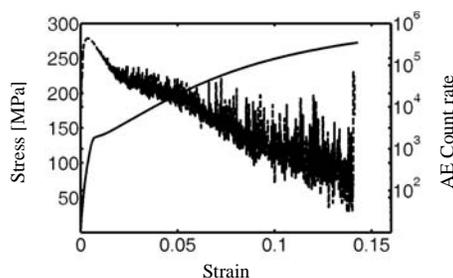
Fig. 4. Characteristic true stress vs. true strain curve (—) and AE (---) for high-pressure die-cast AS21X.
