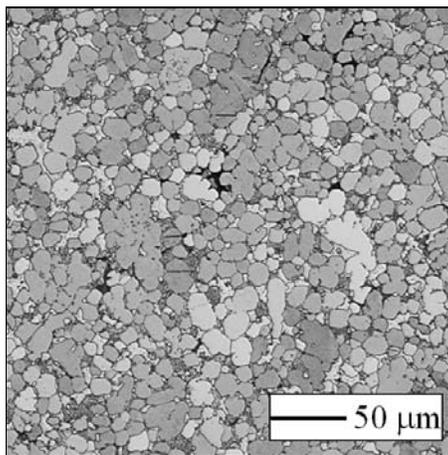
Fig. 2. Microstructure of the high-pressure die-cast AS21X alloy.
