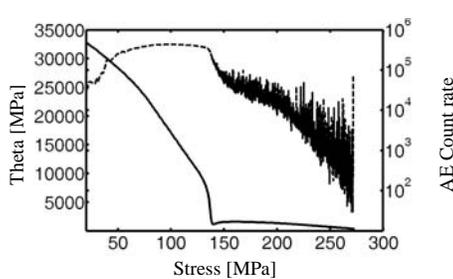
Fig. 6. Strain hardening rate vs. stress (—) and AE (---) for high-pressure die-cast AS21X.
