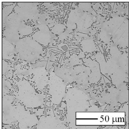
Fig. 1. Microstructure of the squeeze-cast AS21X alloy.
