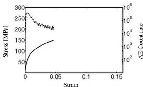
Fig. 3. Typical true stress vs. true strain (—) and AE (---) curves for squeeze-cast AS21X.
