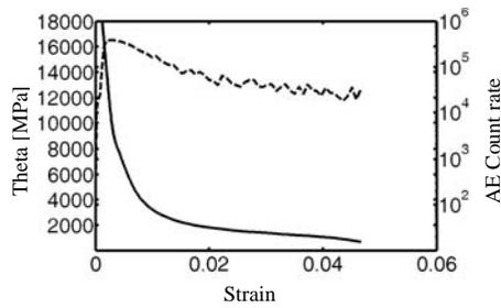
Fig. 7. Strain hardening rate vs. strain (—) and AE (---) for squeeze-cast AS21X.
