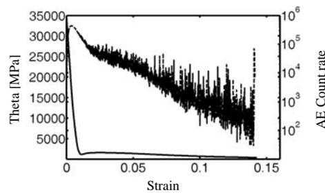
Fig. 8. Strain hardening rate vs. strain (—) and AE (---) for high-pressure die-cast AS21X.
