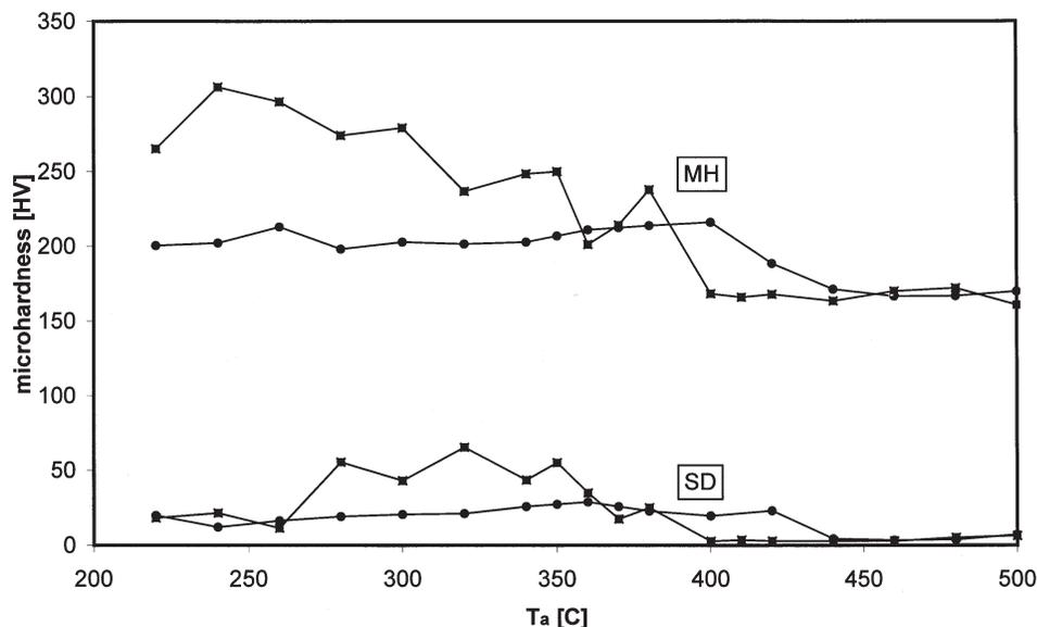
Fig. 3. Temperature dependence of microhardness (MH) and standard deviation (SD) of measured MH-values for a CuAu sample isochronally cooled using temperature program #1 (●) and #2 (■), respectively – see the text. The full lines serve as a guide for the eye.
