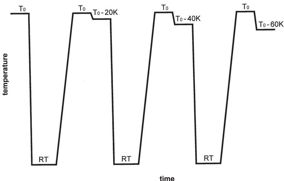
Fig. 2. Schema of the temperature program #2 ( $T_0 = 500^\circ\text{C}$ ,  $\Delta T = 20\text{ K}$ ,  $\Delta t = 10$  minutes).
