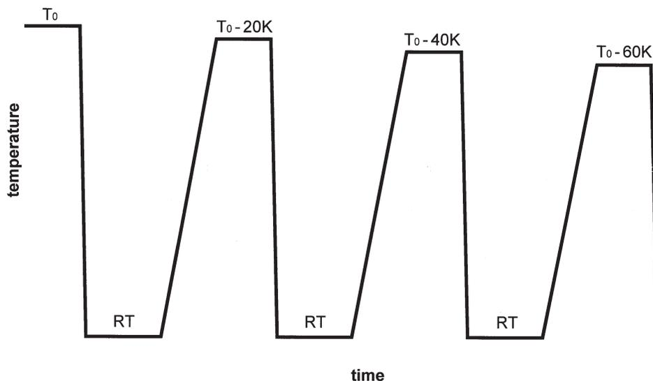
Fig. 1. Schema of a conventional isochronal cooling (temperature program #1) from  $T_0 = 500\text{ °C}$ ; ( $\Delta T = 20\text{ K}$ ,  $\Delta t = 10\text{ minutes}$ ).
