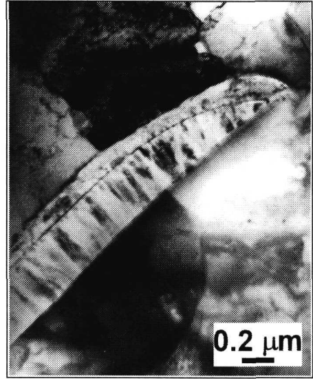
Fig. 8. \gamma - \text{Al}_2\text{O}_3 oxide inclusion in the microstructure of NiCrAlY coating isothermally exposed at 850°C for 100 hours (TEM, bright field image).
