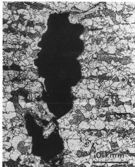
Fig. 6. Detail of the cavity formed in copper disc impacted by a low-velocity projectile (gas gun test). In this test the strain rate approaches the ones encountered during some forming processes.
