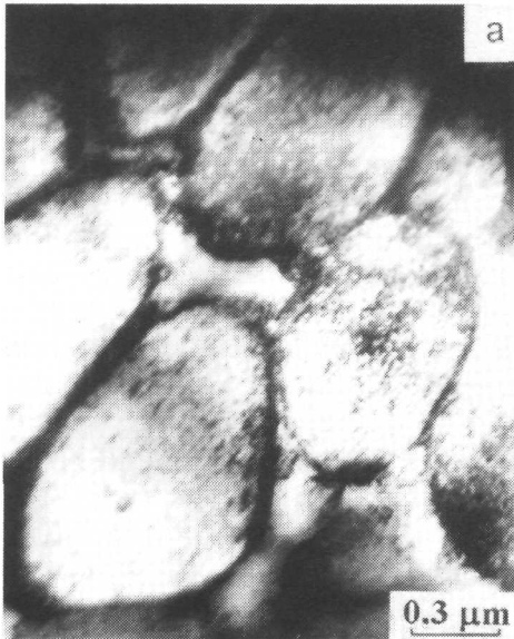
Fig. 6a. Microstructure of NiCrAlY powders (TEM, bright field image).
