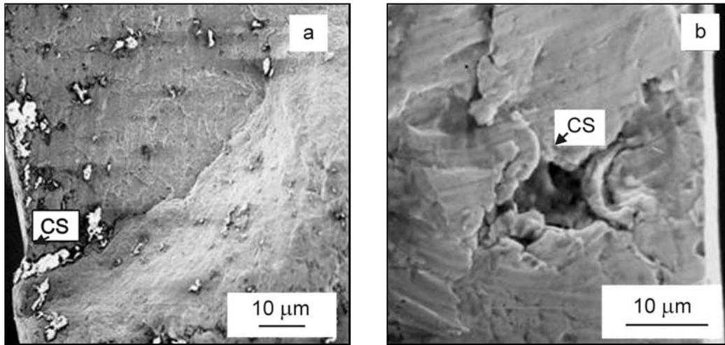
Fig. 7. SEM fractographs of plain fatigue specimens at (a) untreated at  $\sigma = 402$  MPa and (b) induction hardened at  $\sigma = 442$  MPa; CS: Crack initiation site.
