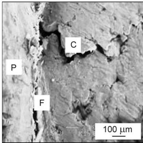
Fig. 9. SEM fractograph of the stick of contact pad to untreated fretting fatigue specimen at a contact pressure of 200 MPa; P: Pad, C: Crack step, F: Fretted surface.
