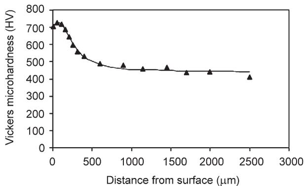
Fig. 3. Relationship between hardness and distance from fretting surface.
