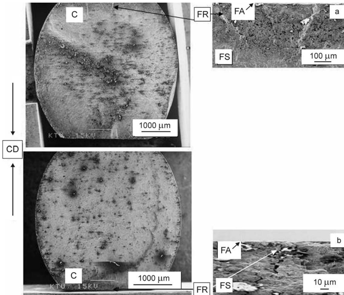
Fig. 8. SEM fractographs of fretting fatigue specimens at (a) untreated at  $\sigma = 405$  MPa and (b) induction hardened at  $\sigma = 387$  MPa; FA: Fretted area, FS: Fracture surface, CD: Crack growth direction, C: Crack step, FR: Fracture initiation region.
