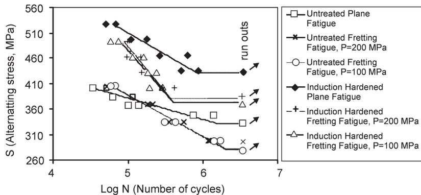
Fig. 4. S-N curves obtained from plain fatigue tests and fretting fatigue tests of AISI 1045 steel.
