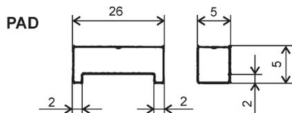
Fig. 1. Schematic drawings of fretting fatigue specimen and fretting pad in millimetres.
