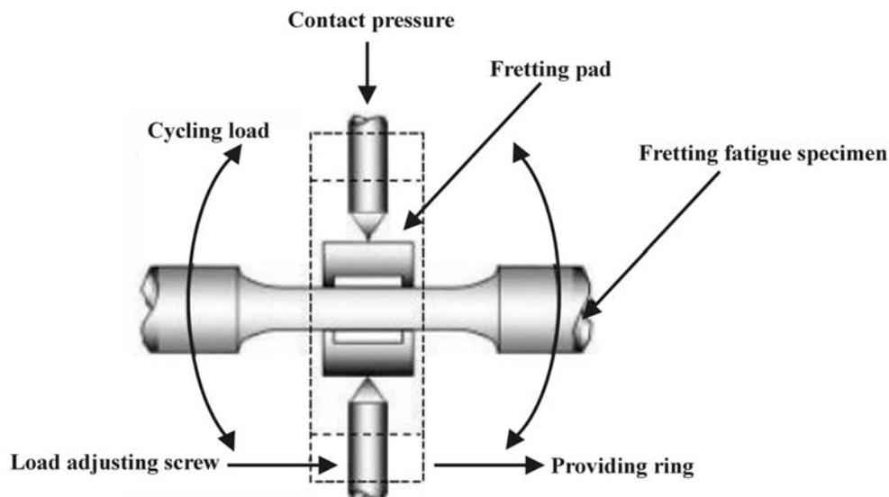
Fig. 2. Schematic drawing of the fretting fatigue testing system in a rotating bending machine.
