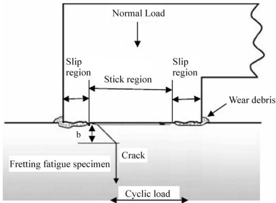
Fig. 6. Schematic drawing of fretting damage;  $b$ : depth of fracture initiation zone site.
