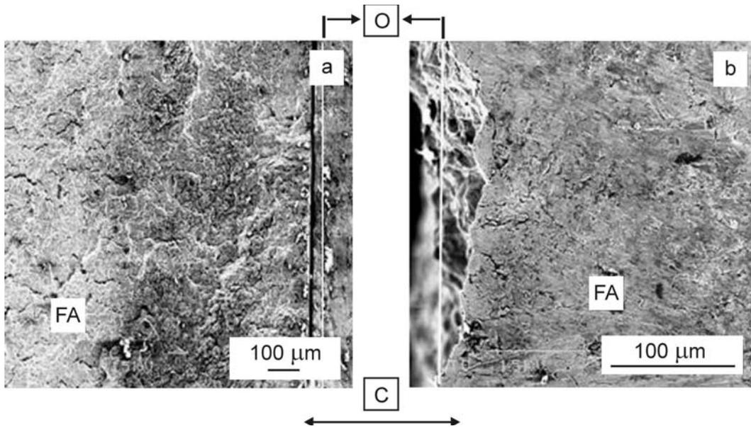
Fig. 5. SEM fractographs of fretted areas of fretting fatigue specimens at (a) untreated at  $P = 100$  MPa and (b) untreated at  $P = 200$  MPa; FA: Fretted area, O: Outer edges, C: Cyclic load direction.
