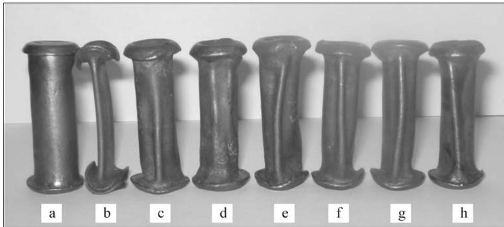
Fig. 4. The deformation of the flexible container under applied pressures: (a) before pressing, (b) empty pressing (20 MPa), (c) 100 MPa, (d) 200 MPa, (e) 300 MPa, (f) 400 MPa, (g) 500 MPa, (h) 600 MPa.
