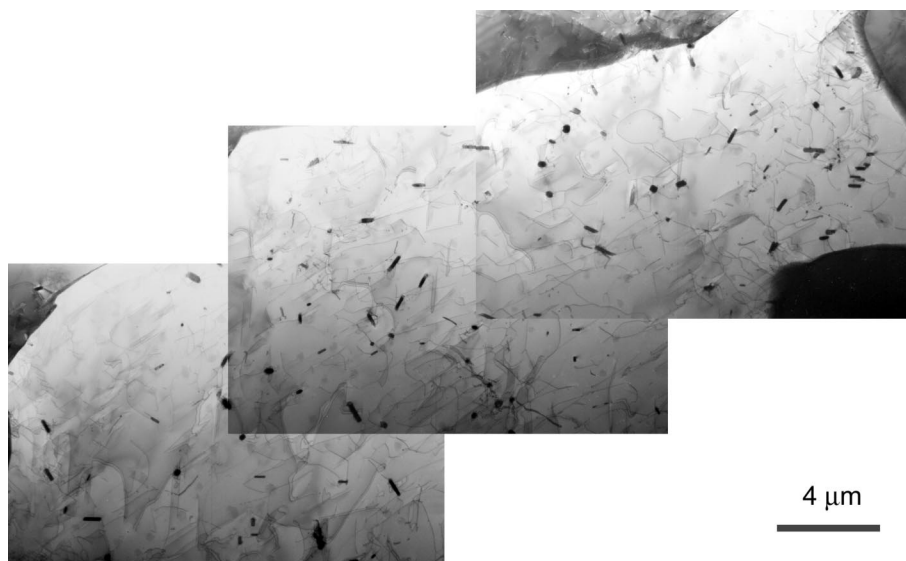
Fig. 4. Microstructure of the sample after creep test at 600°C.
