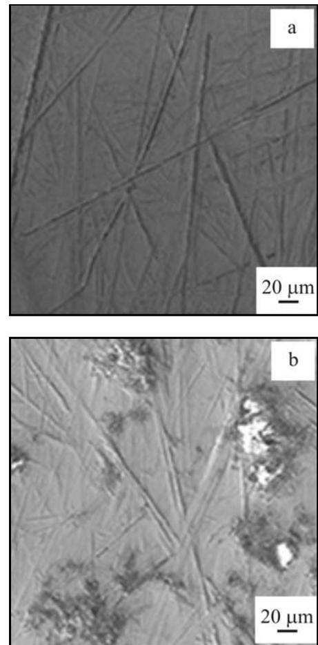
Fig. 6. Worn out surface of DCT20 (a) and CHT20 (b) (800×).
