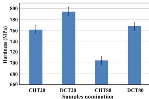
Fig. 4. Vickers hardness of the 100Cr6 low alloy steel samples.
