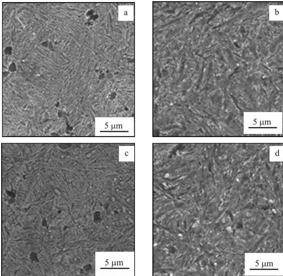
Fig. 2. SEM micrographs of the carbides in the 100Cr6 low alloy steel: CHT80 (a), CHT20 (b), DCT80 (c) and DCT20 (d) (6000×).
