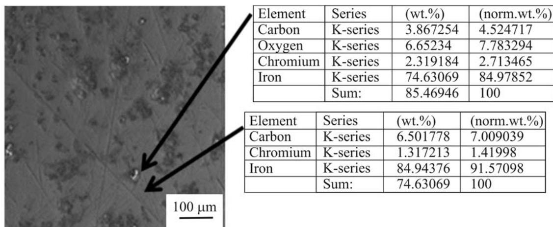
Fig. 7. EDX analysis of the worn-out surface of the CHT20 sample after 1000 m sliding.
