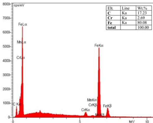
Fig. 3. EDX analysis of the carbide in the 100Cr6 samples and its composition.
