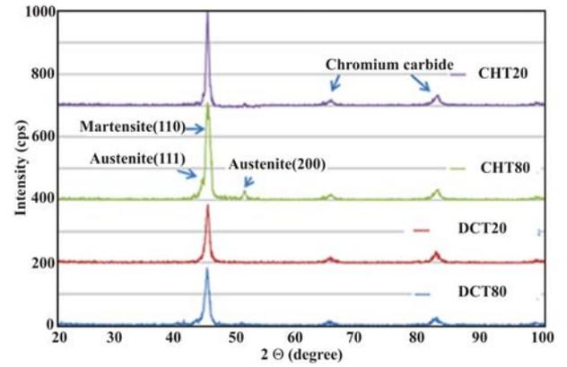
Fig. 1. XRD diagram of the 100Cr6 low alloy steel.
