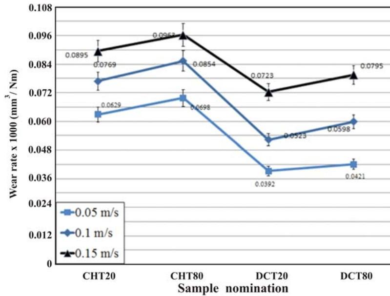
Fig. 5. Wear rate of samples at different sliding speeds of 0.05, 0.1 and 0.15 m s<sup>-1</sup> under 220 N normal load in pin-on-disk wear test.
