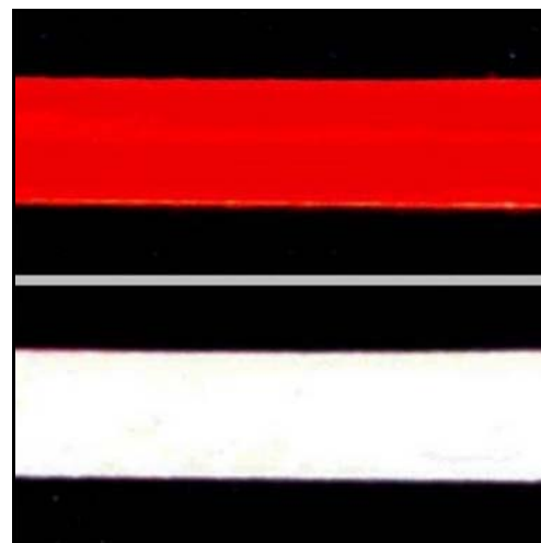
Fig. 5. Liquid penetrant examination result of an AA6061-O joint.
