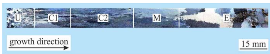
Fig. 1. OM showing the typical macrostructure of longitudinal section of sample prepared by power down technique in Bridgman type apparatus: U – non-melted part, C 1 – columnar zone formed at a growth rate of V = 2.78 \times 10^{-4} \text{ m s}^{-1} and temperature gradient of G_L = 5.5 \times 10^3 \text{ K m}^{-1} , C 2 – columnar zone formed at a cooling rate of v = 0.5 \text{ K s}^{-1} , M – mixed columnar and equiaxed zone and E – equiaxed zone.
