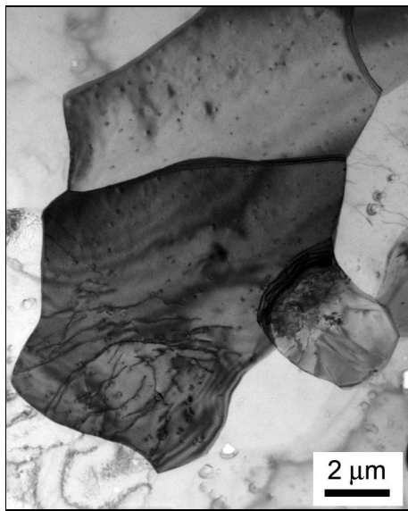
Fig. 5. Bright field TEM micrograph of recrystallized grains in hot-rolled AZ31 (OF) preheated at 325 °C ( \mathbf{g} = (10\bar{1}0) , \mathbf{B} = [0001] ).
