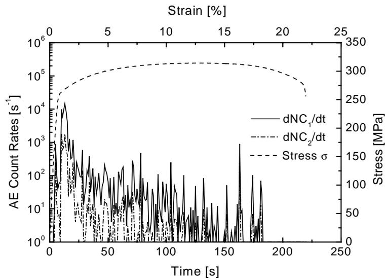
Fig. 3. Stress-strain and AE count rates-time curves for extruded AZ31 alloy with grain size 4  $\mu\text{m}$ .
