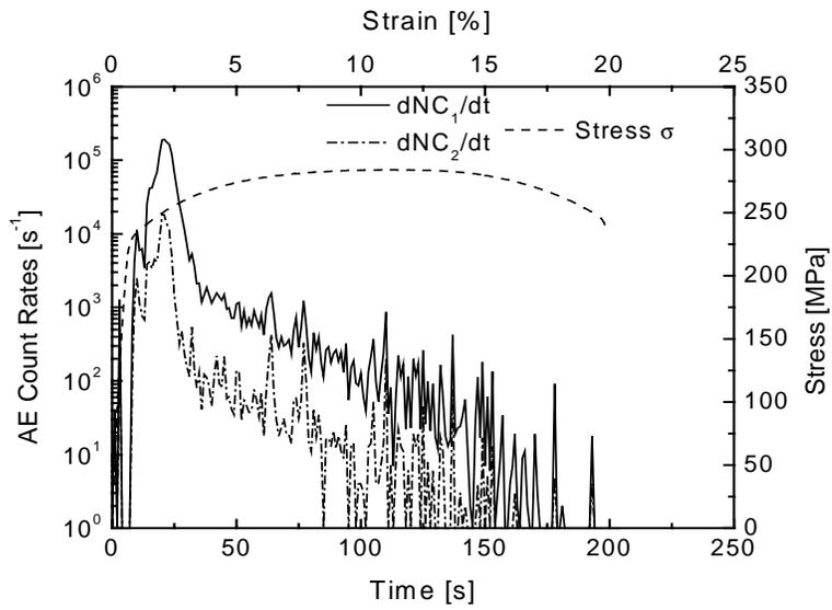
Fig. 4. Stress-strain and AE count rates-time curves for extruded AZ31 alloy with grain size  $6 \mu\text{m}$ .
