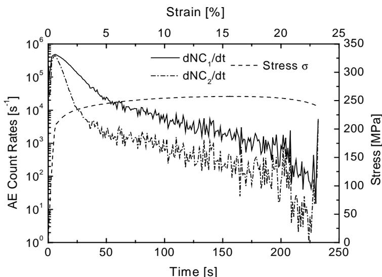
Fig. 6. Stress-strain and AE count rates-time curves for extruded AZ31 alloy with grain size 22  $\mu\text{m}$ .
