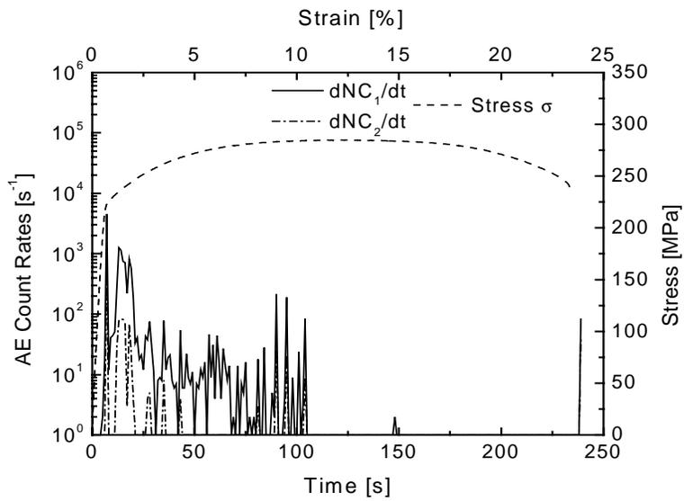
Fig. 5. Stress-strain and AE count rates-time curves for extruded AZ31 alloy with grain size  $8 \mu\text{m}$ .
