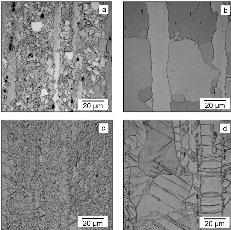
Fig. 1. Micrographs of extruded AZ31 alloy: (a) hydrostatic, grain size  $4\ \mu\text{m}$ , (b) indirect, grain size  $22\ \mu\text{m}$ , (c) hydrostatic, grain size  $4\ \mu\text{m}$ , after tensile testing, (d) indirect, grain size  $22\ \mu\text{m}$ , after tensile testing.
