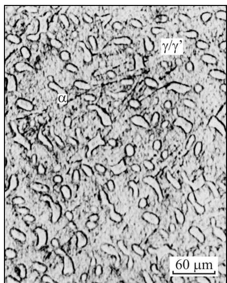
Fig. 1. Optical micrograph showing the typical as-cast microstructure of the Alloy 1.
