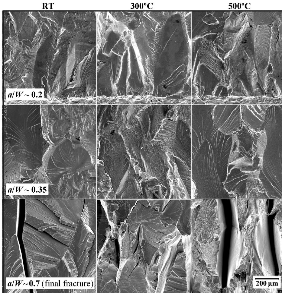
Fig. 2. Fracture surfaces at room temperature (RT) and at elevated temperatures (300, 500 °C) at the start of the fatigue crack growth (near the pre-crack,  $a/W \sim 0.2$ ), during the fatigue crack growth ( $a/W \sim 0.35$ ) and in the area of final fracture ( $a/W \sim 0.7$ ).
