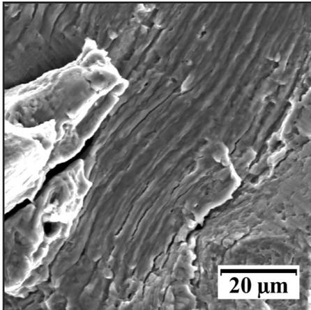
Fig. 5. Ductile striations formed on the fracture surface at 300 °C.
