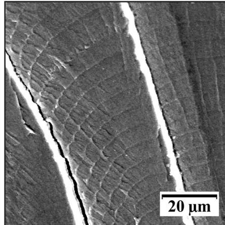
Fig. 6. Brittle striations covering the cleavage facets at 500 °C.
