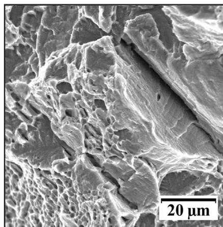
Fig. 8. Ductile dimples on the final fracture surface at 500 °C.
