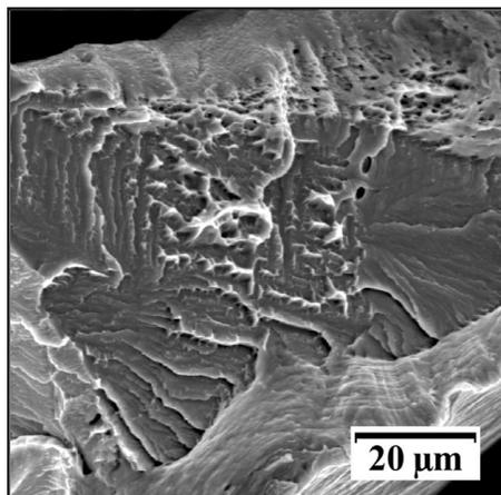
Fig. 7. Signs of increasing plastic deformation during the final fracture at 300 °C.
