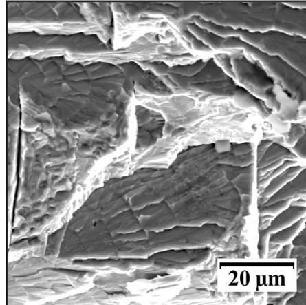
Fig. 4. Cyclic cleavage on fracture surfaces at room temperature.
