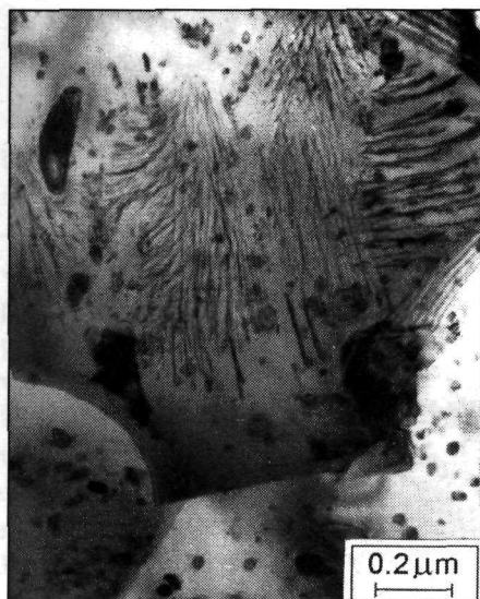
Fig. 6. Microstructure of the slightly over-aged Zr-rich Al-Zr-Ti alloy ( x = 0.5 ), T = 650 K, t = 500 hours.
