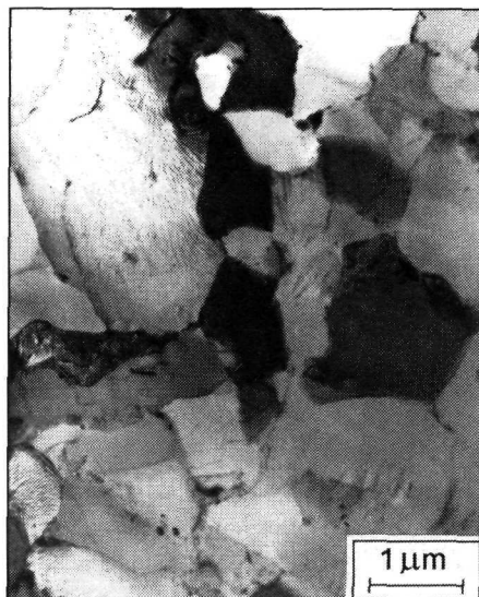
Fig. 4. Microstructure of the peak-aged binary Al-Zr alloy, T = 600 K, t = 10 hours.
