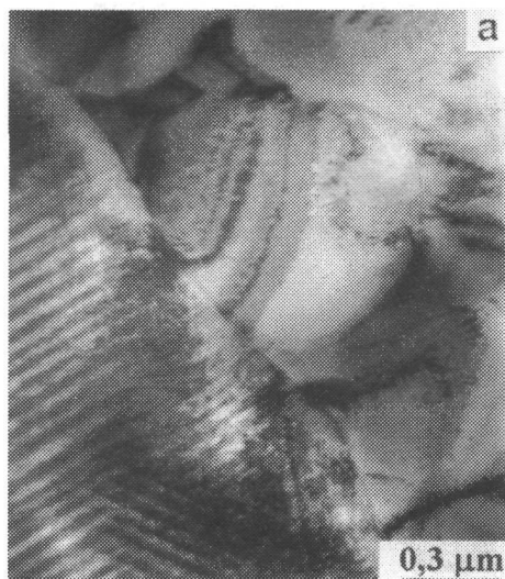
Fig. 7a. A bright field transmission electron micrograph showing the martensitic and \gamma/\gamma' phases in the structure of NiCrAlY powders.
