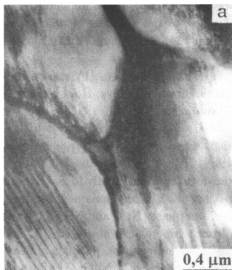
Fig. 8a. A bright field transmission electron micrograph showing the NiAl-martensite and \gamma phases in the structure of NiCrAlY powders.
