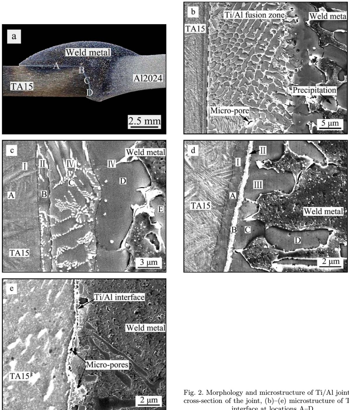
Fig. 2. Morphology and microstructure of Ti/Al joint: (a) cross-section of the joint, (b)–(e) microstructure of Ti/Al interface at locations A–D.
