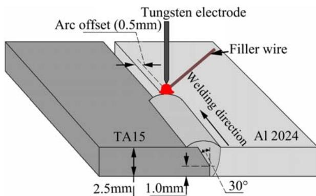
Fig. 1. Schematic drawing of TIG welding.
