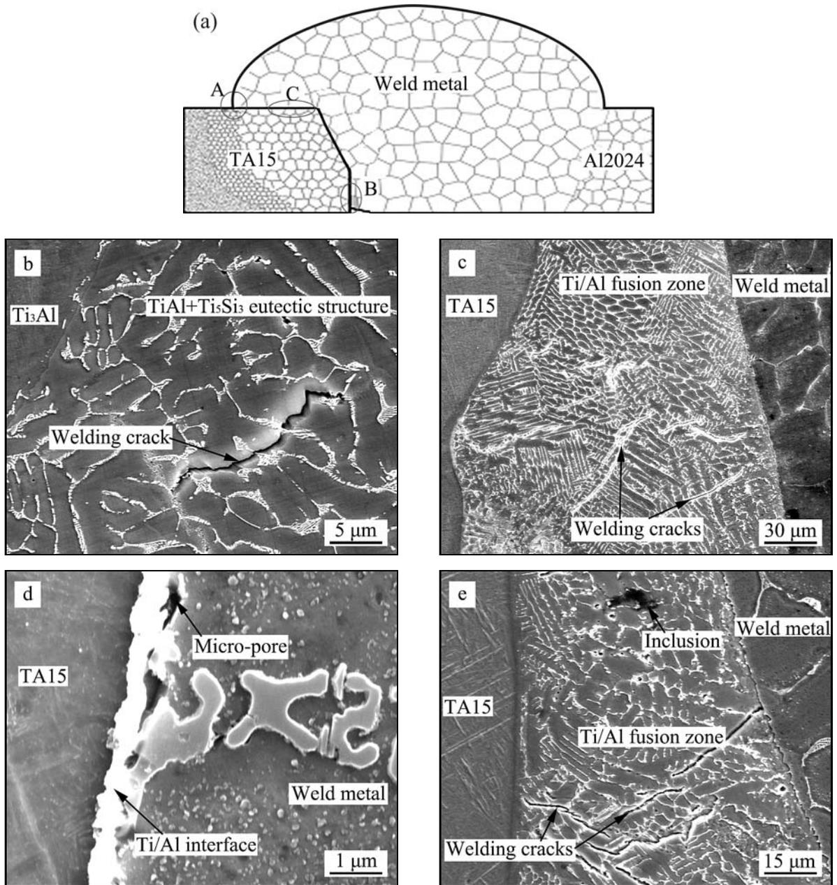
Fig. 4. Initiation of cracks near Ti/Al interface: (a) schematic diagram of Ti/Al joint, (b) crack in Ti-Al IMCs, (c)–(e) microstructure of Ti/Al interfaces at locations A–C.
