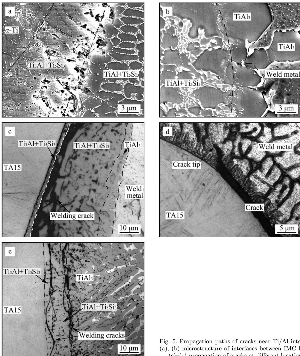
Fig. 5. Propagation paths of cracks near Ti/Al interface: (a), (b) microstructure of interfaces between IMC layers, (c)–(e) propagation of cracks at different locations.
