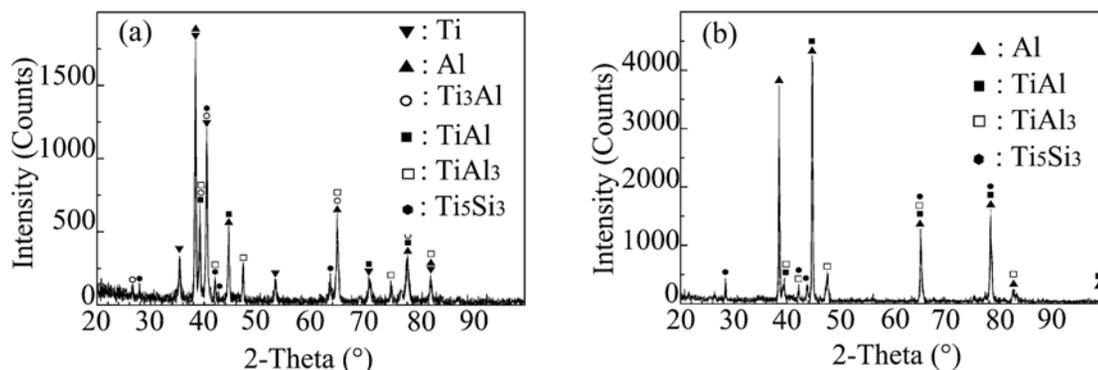
Fig. 3. X-ray diffraction profiles of the Ti/Al interface: (a) Ti side, (b) Al side.
